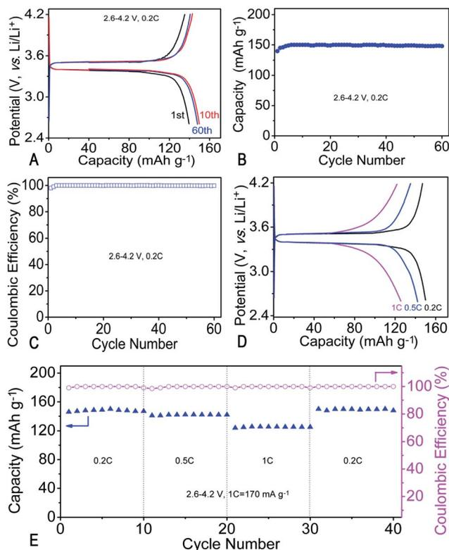
Fig. 3 Electrochemical performances of Li/MIEM/LiFePO<sub>4</sub> cells at 20 °C: (A) charge/discharge profiles for the 1st, 10th and 60th cycle, (B) discharge capacity and (C) Coulombic efficiency during cycling at 0.2C; (D) representative charge/discharge voltage profiles at current densities from 0.2C to 1C; (E) capacity and Coulombic efficiency during cycling at current densities from 0.2C to 1C (each for ten successive cycles).
