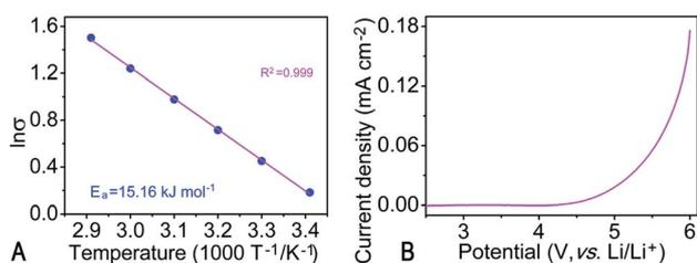
Fig. 2 (A)  $\ln \sigma$  dependence on temperature ( $T$ ) of the resulted monolithic ionogel electrolyte membrane (MIEM) ( $\ln \sigma$  vs.  $T^{-1}$  plot); (B) linear sweep voltammograms (LSV) of the MIEM.
