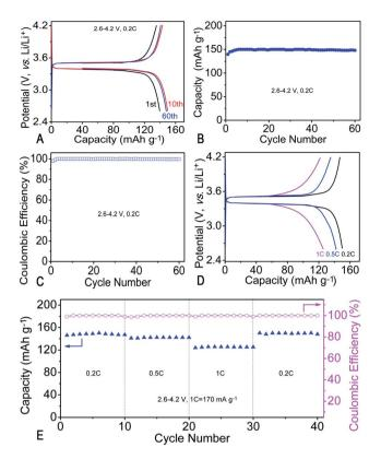
Fig. 3 Electrochemical performances of Li/MIEM/LiFePO $_4$  cells at 20 °C: (A) charge/discharge profiles for the 1st, 10th and 60th cycle, (B) discharge capacity and (C) Coulombic efficiency during cycling at 0.2C; (D) representative charge/discharge voltage profiles at current densities from 0.2C to 1C; (E) capacity and Coulombic efficiency during cycling at current densities from 0.2C to 1C (each for ten successive cycles).
