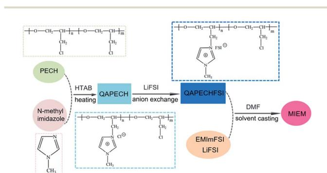
**Scheme 1** Schematic diagram for the preparation of the quaternary ammonium poly (epichlorohydrin) with the bis-(fluorosulfonyl) imide side chain (QAPECHFSI) and resulted monolithic ionogel electrolyte membrane (MIEM) (HTAB: hexadecyl trimethyl ammonium bromide; LiFSI: lithium bis (fluorosulfonyl)imide; EMImFSI: 1-ethyl-3-methylimidazolium bis-(fluorosulfonyl)-imide; DMF: *N,N*-dimethylformamide).
