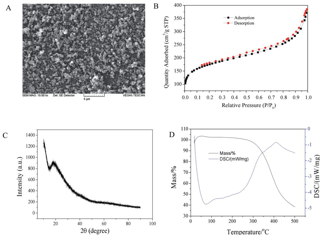
Fig. 4 SEM photo (A), N<sub>2</sub> adsorption–desorption isotherms (B), XRD pattern (C), and TGA curve of MIPs-POSS coating (C3).
