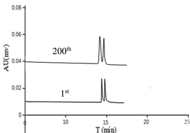
Fig. 7 Electropherograms of DL-His on c3 column of the 1st and 200th running. Conditions: capillary, 75  $\mu$ m i.d. (375  $\mu$ m o.d.), 60.0 cm total length and 50.0 cm effective length; separation voltage, 15 kV; detection wavelength, 214 nm; injection, 0.5 psi  $\times$  3 s; buffer, 20 mmol L<sup>-1</sup> phosphate (pH 7.4).
