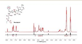
Fig. 1 Remdesivir molecular structure and its normal <sup>1</sup>H NMR signal in the methanol-d<sub>4</sub> solvent (black spectrum). Hyperpolarized signals from remdesivir after SABRE in the presence of 130 G external magnetic field in the methanol-d<sub>4</sub> solvent (red spectrum).
