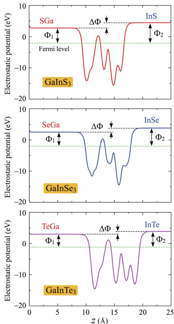
Fig. 6 Planar electrostatic potential of the Janus GaInX<sub>3</sub> (X = S, Se, Te) single-layers with dipole correction.  $\Delta\Phi$  is the difference in the vacuum levels between the XGa and InX sides.
