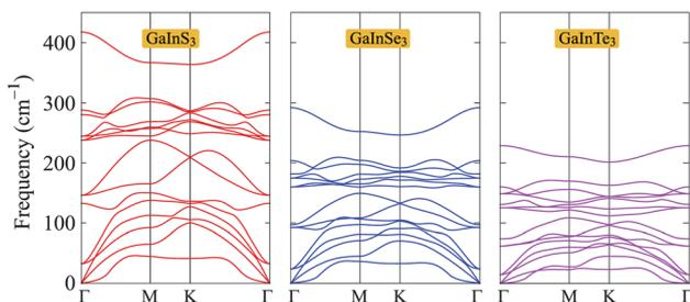
Fig. 2 Phonon dispersions of GaInS<sub>3</sub>, GaInSe<sub>3</sub>, and GaInTe<sub>3</sub> single-layers.
