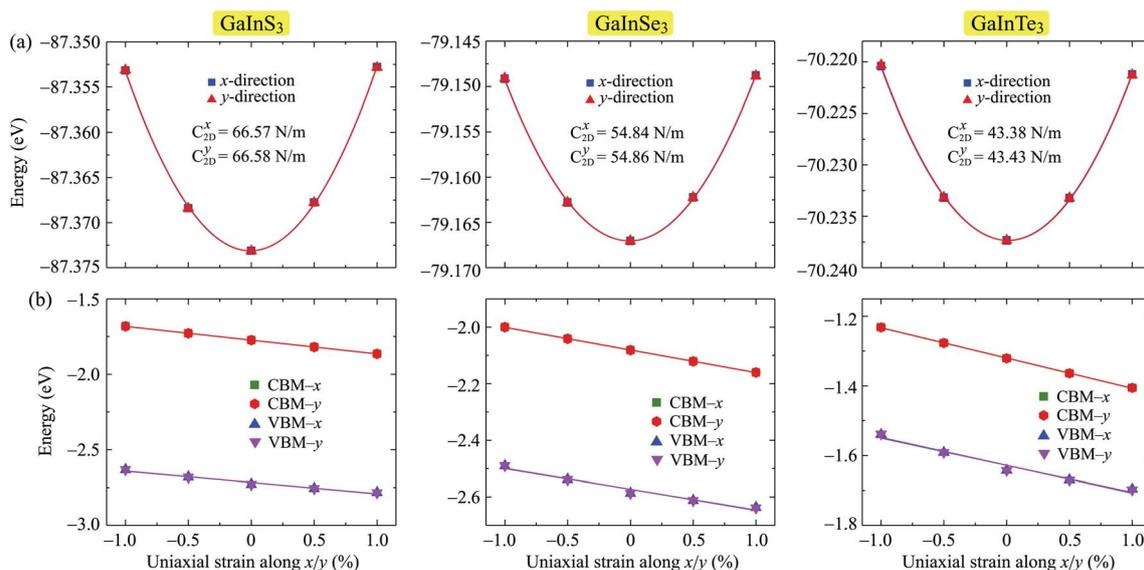
**Fig. 7** Strain-dependent total energy (a) and band-edge positions (b) of GaInX<sub>3</sub> single-layers along two transport directions  $x$  and  $y$ .
