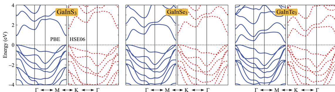
Fig. 4 Band structures along the high-symmetry direction  $\Gamma$ - $M$ - $K$ - $\Gamma$  of Janus  $\text{GaInX}_3$  (X = S, Se, Te) single-layers at the PBE (solid lines) and HSE06 (dashed lines) levels.
