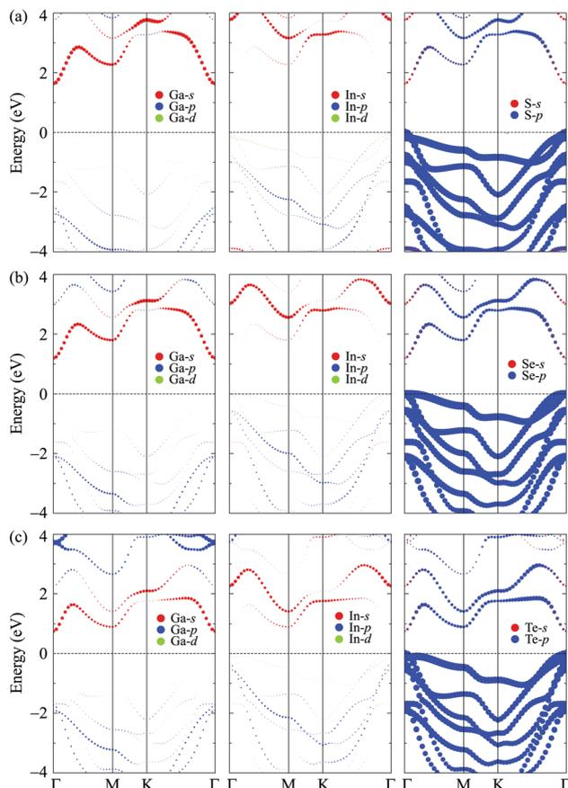
Fig. 5 Weighted bands of GaInS<sub>3</sub> (a), GaInSe<sub>3</sub> (b), and GaInTe<sub>3</sub> (c) single-layers at the HSE06 level.
