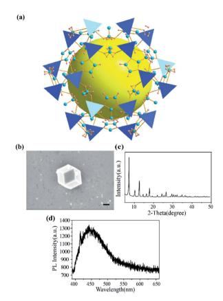
Fig. 1 (a) Crystal structure of ZIF-8: Zn (polyhedral), C (blue sphere), and H (pink sphere). The largest sphere (yellow) represents the largest van der Waals spheres that would fit in the cavities without touching the framework. (b) TEM images of ZIF-8 (scale bar: 300 nm). (c) XRD pattern of synthesized ZIF-8. (d) Fluorescence spectra of ZIF-8 under excitation at 375 nm.
