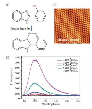
Fig. 2 (a) Chemical structure of HPBI and proton transfer of HPBI. (b) Typical STM image of HPBI on Au (111) ( $10 \times 10 \text{ nm}^2$ , -2.7 V, 10 pA). (c) Fluorescence spectra of HPBI with different concentrations under excitation at 375 nm.
