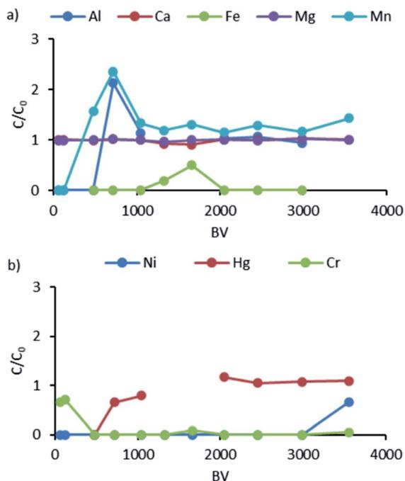
Fig. 5 Breakthrough curves for K1: (a) data for Al, Ca, Fe, Mg, and Mn; (b) data for Ni, Hg, and Cr.
