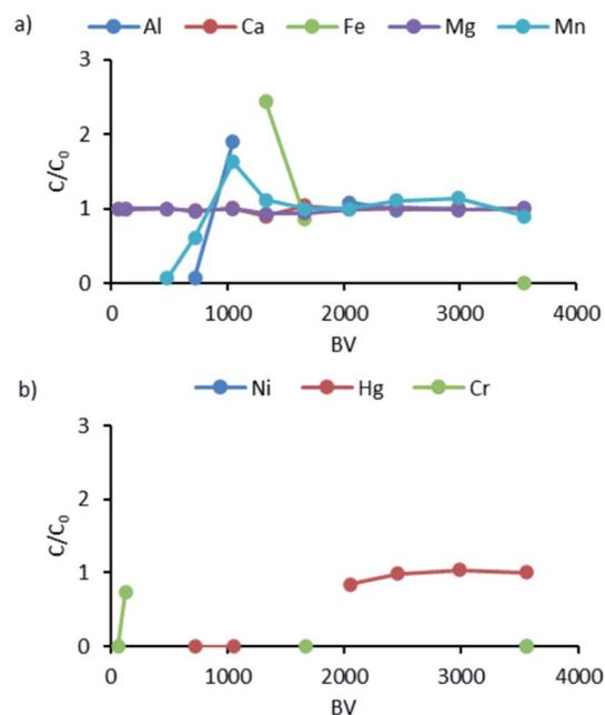
Fig. 6 Breakthrough curves for K2: (a) data for Al, Ca, Fe, Mg, and Mn; (b) data for Ni, Hg, and Cr.
