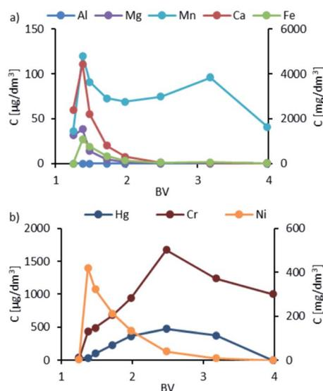
Fig. 8 Elution profiles of K1: (a) data for Al and Mn in  $\mu\text{g dm}^{-3}$ , and Mn, Ca, and Fe in  $\text{mg dm}^{-3}$ ; (b) data for Hg and Cr in  $\mu\text{g dm}^{-3}$  and Ni in  $\text{mg dm}^{-3}$ .
