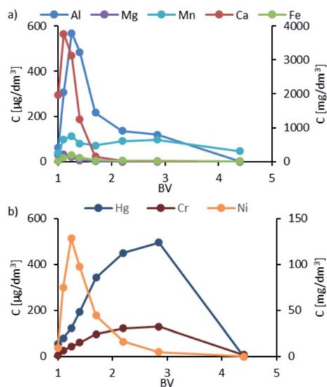
Fig. 9 Elution profiles of K2: (a) data for Al and Mn in  $\mu\text{g dm}^{-3}$ , and Mn, Ca, and Fe in  $\text{mg dm}^{-3}$ ; (b) data for Hg and Cr in  $\mu\text{g dm}^{-3}$  and Ni in  $\text{mg dm}^{-3}$ .
