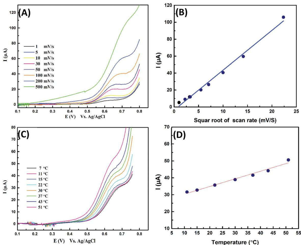
Fig. 5 (A) LSVs response of the nano-Cu/Cu-wire in 0.075 mg L<sup>-1</sup> NaOH solution containing 75 mg L<sup>-1</sup> glycine (B) linear relationship between the oxidation current and square root of scan rate, (C) examine the effect of temperature on the oxidation response, and (D) the linear plot between the oxidation current and temperature.
