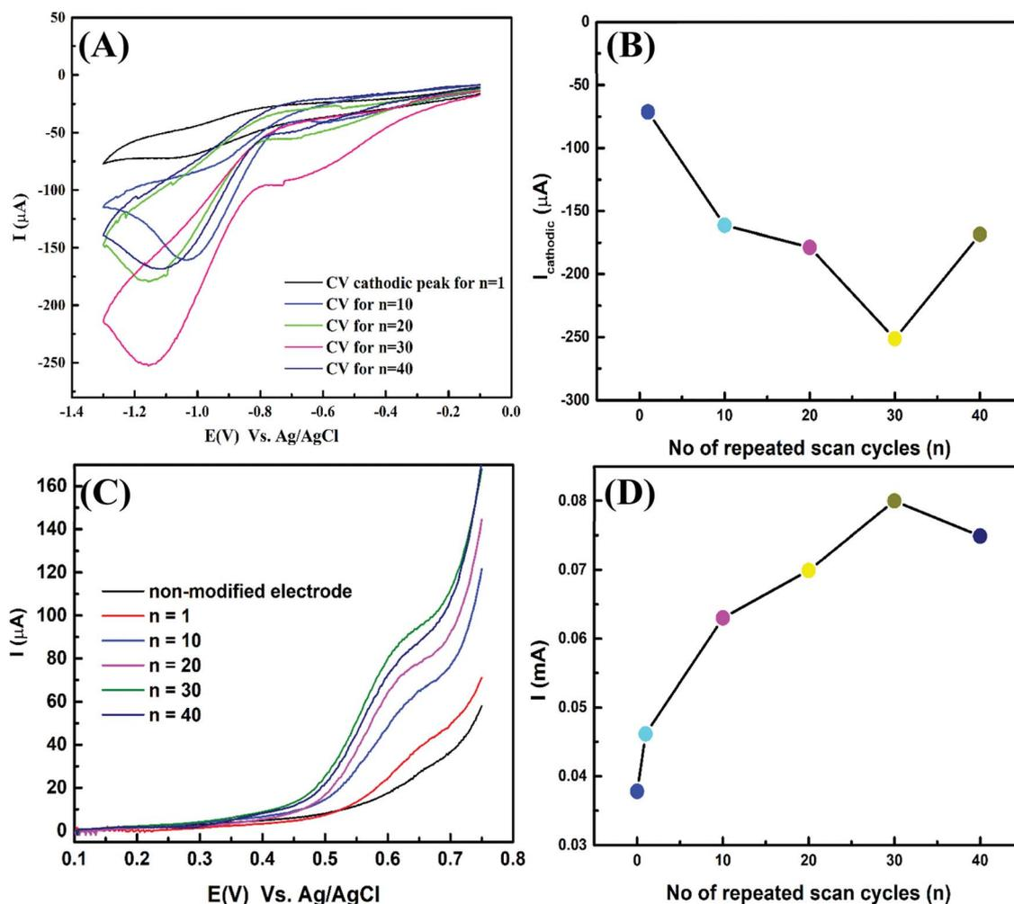
Fig. 4 (A) FSCV deposition of Cu film at different ( $n$ ); (B) the relation between ( $n$ ) and the cathodic peak current ( $I$ ,  $\mu\text{A}$ ) obtained from CV, (C) LSVs in  $75 \text{ mg L}^{-1}$  gly/0.075 M NaOH for nano-Cu sensors prepared at different ( $n$ ) at  $25^\circ\text{C}$  and (D) the relation between ( $n$ ) and the anodic peak current ( $I$ , mA) obtained from LSV.
