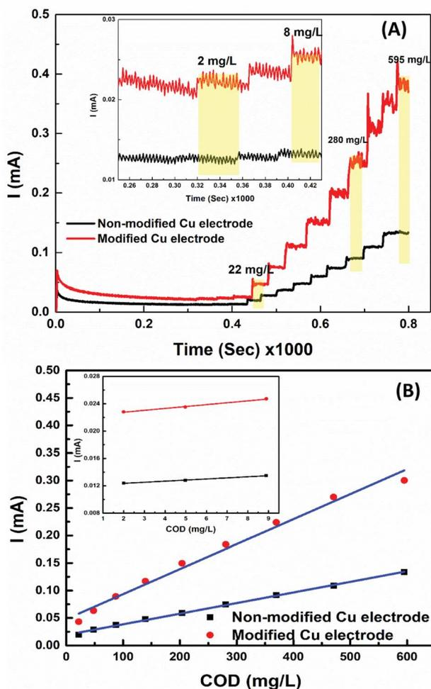
Fig. 6 (A) ( $I-t$ ) response curves of modified and non-modified Cu electrodes at different COD concentrations; inset of (A) is the response at lower COD concentrations. (B) Calibration curves of modified and non-modified Cu electrodes; inset of (B) is at lower COD concentrations.
