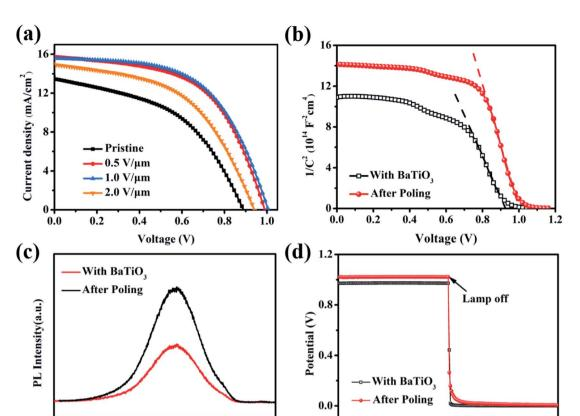
Fig. 7 (a) J-V characteristic curves of the BaTiO<sub>3</sub>@MAPbl<sub>3</sub>-based C-PSCs treated with different voltage polarization. (b) Mott–Schottky curves; (c) steady-state PL spectra; and (d) voltage attenuation curves of the BaTiO<sub>3</sub>@MAPbl<sub>3</sub>-based C-PSCs before and after polarization treatment.
