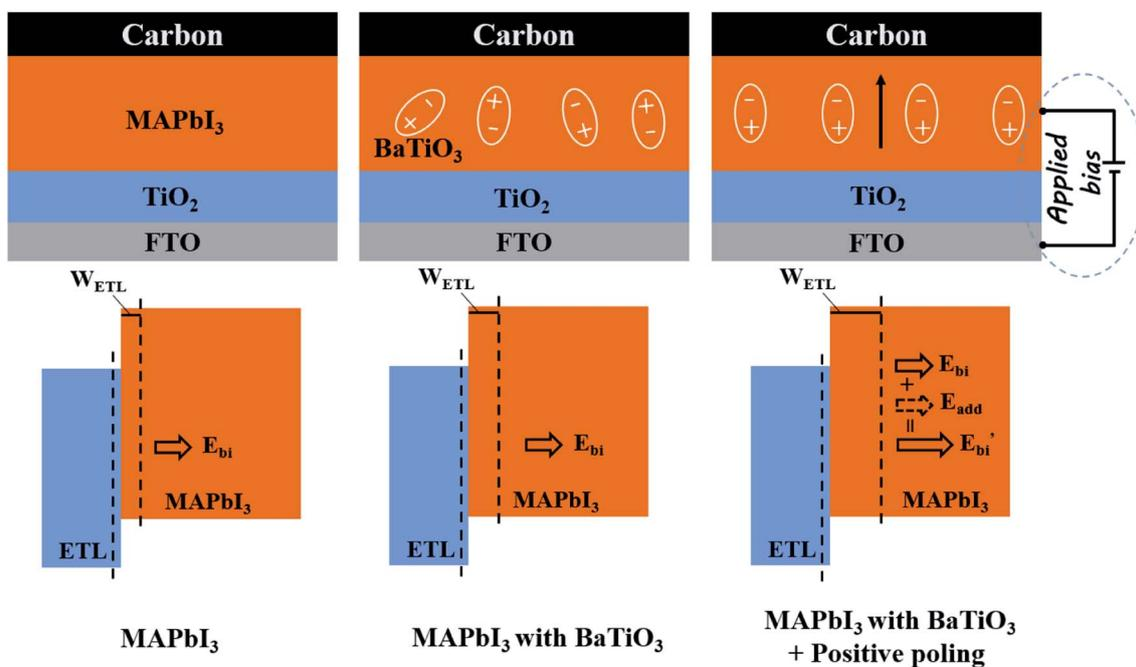
Fig. 9 Performance improvement schematic of the BaTiO<sub>3</sub>@MAPbI<sub>3</sub>-based C-PSCs.
