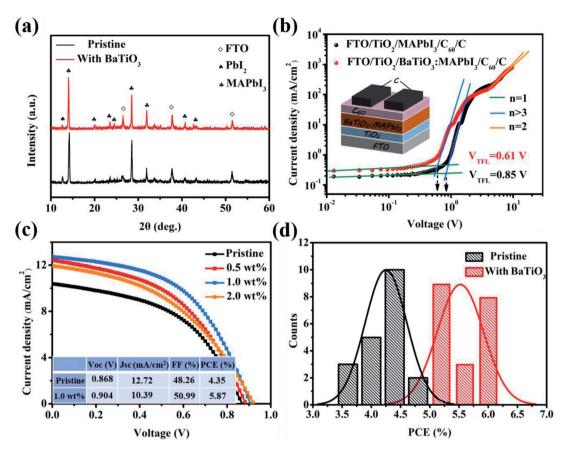
Fig. 4 (a) XRD patterns of MAPbl $_3$  and BaTiO $_3$ :MAPbl $_3$  (b) SCLC tests based on the MAPbl $_3$  and BaTiO $_3$ :MAPbl $_3$  single electronic devices. (c) J-V characteristic curve of C-PSCs prepared with BaTiO $_3$  doped with MAPbl $_3$  at different concentrations. (d) Efficiency statistics of the MAPbl $_3$  and BaTiO $_3$ :MAPbl $_3$ -based C-PSCs.
