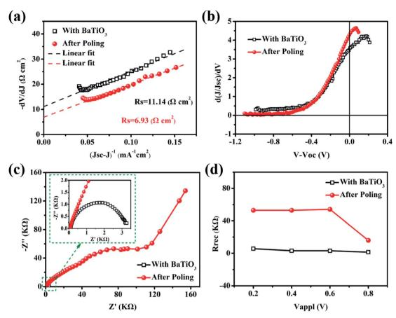
Fig. 8 (a) The relationship curve between -dV/dJ and  $(J_{SC}-J)^{-1}$ . (b) Relationship curve between  $\ln(J_{SC}-J)$  and  $(V+R_SJ)$ . (c) EIS curve. (d)  $R_{rec}$  at different bias of the BaTiO<sub>3</sub>@MAPbl<sub>3</sub>-based C-PSCs before and after polarization treatment.
