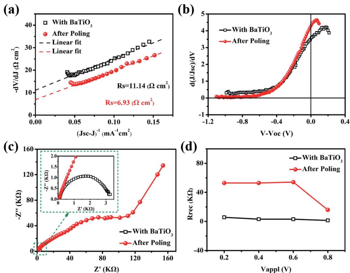
Fig. 8 (a) The relationship curve between  $-dV/dJ$  and  $(J_{SC} - J)^{-1}$ . (b) Relationship curve between  $\ln(J_{SC} - J)$  and  $(V + R_S J)$ . (c) EIS curve. (d)  $R_{rec}$  at different bias of the  $BaTiO_3@MAPbI_3$ -based C-PSCs before and after polarization treatment.
