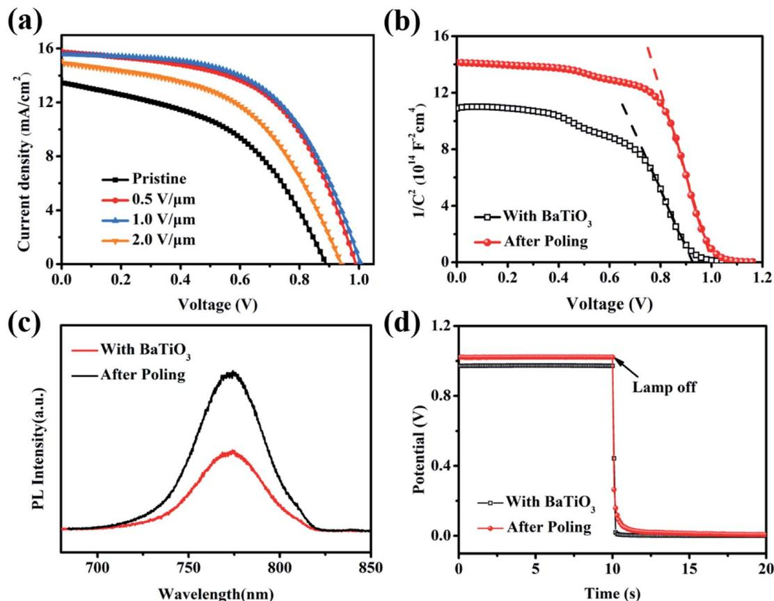
Fig. 7 (a)  $J$ - $V$  characteristic curves of the  $\text{BaTiO}_3$ @ $\text{MAPbI}_3$ -based C-PSCs treated with different voltage polarization. (b) Mott-Schottky curves; (c) steady-state PL spectra; and (d) voltage attenuation curves of the  $\text{BaTiO}_3$ @ $\text{MAPbI}_3$ -based C-PSCs before and after polarization treatment.
