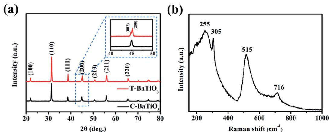
Fig. 2 (a) XRD patterns of BaTiO<sub>3</sub> powders before and after sintering. (b) Raman spectrum of BaTiO<sub>3</sub> powders after sintering.
