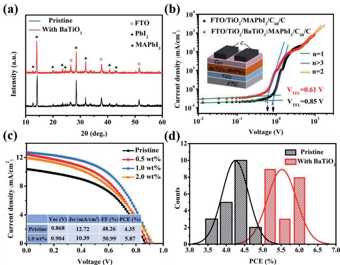
Fig. 4 (a) XRD patterns of MAPbI<sub>3</sub> and BaTiO<sub>3</sub>:MAPbI<sub>3</sub>. (b) SCLC tests based on the MAPbI<sub>3</sub> and BaTiO<sub>3</sub>:MAPbI<sub>3</sub> single electronic devices. (c) *J*-*V* characteristic curve of C-PSCs prepared with BaTiO<sub>3</sub> doped with MAPbI<sub>3</sub> at different concentrations. (d) Efficiency statistics of the MAPbI<sub>3</sub> and BaTiO<sub>3</sub>:MAPbI<sub>3</sub>-based C-PSCs.
