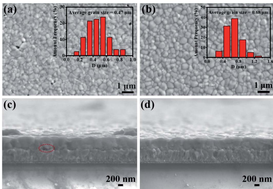
Fig. 3 FE-SEM images of (a) FTO/TiO<sub>2</sub>/MAPbI<sub>3</sub> and (b) FTO/TiO<sub>2</sub>/BaTiO<sub>3</sub>:MAPbI<sub>3</sub>. Cross section images of (c) FTO/TiO<sub>2</sub>/MAPbI<sub>3</sub> and (d) FTO/TiO<sub>2</sub>/BaTiO<sub>3</sub>:MAPbI<sub>3</sub>. The insets in (a) and (b) are the grain size distributions of the corresponding samples.
