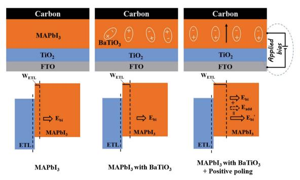
Fig. 9 Performance improvement schematic of the BaTiO<sub>3</sub>@MAPbI<sub>3</sub>-based C-PSCs.
