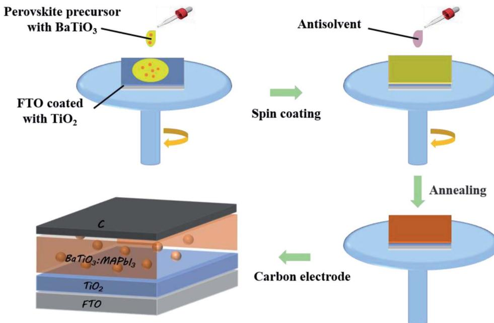
Fig. 1 BaTiO<sub>3</sub>@MAPbI<sub>3</sub> composite film and the device preparation processes.
