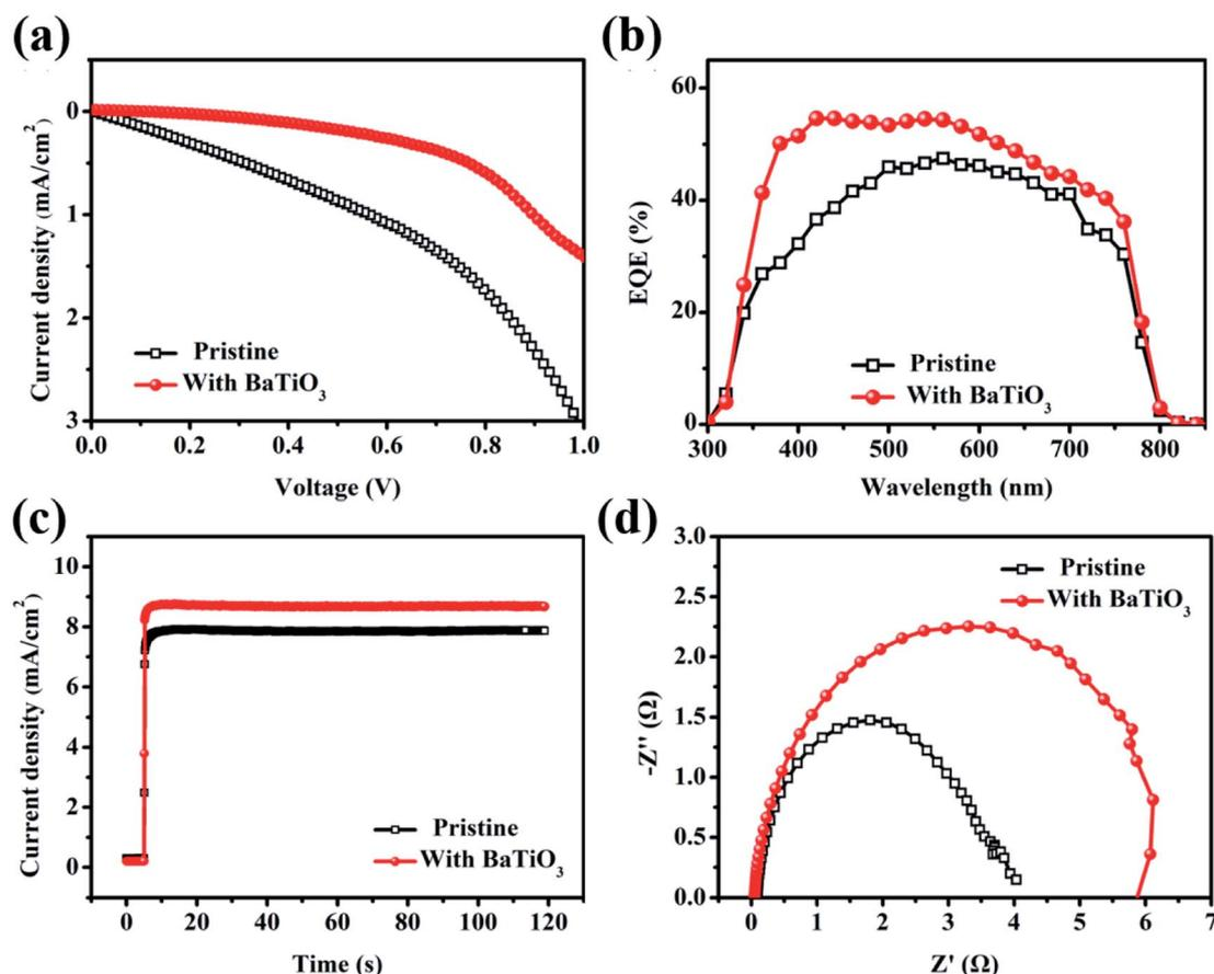
Fig. 5 (a) Dark current curve, (b) EQE curve, and (c) steady-state output current curve at the maximum power point. (d) Impedance diagram of the MAPbI<sub>3</sub> and BaTiO<sub>3</sub>@MAPbI<sub>3</sub>-based C-PSCs.
