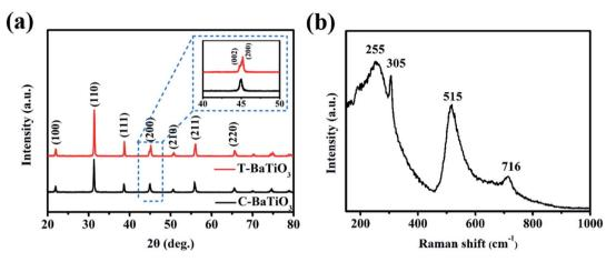
Fig. 2 (a) XRD patterns of BaTiO<sub>3</sub> powders before and after sintering. (b) Raman spectrum of BaTiO<sub>3</sub> powders after sintering.
