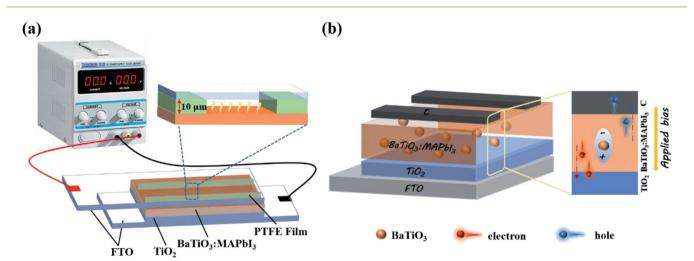
(a) A diagram of the thin film polarization device, (b) Polarization schematic diagram of the C-PSCs.
