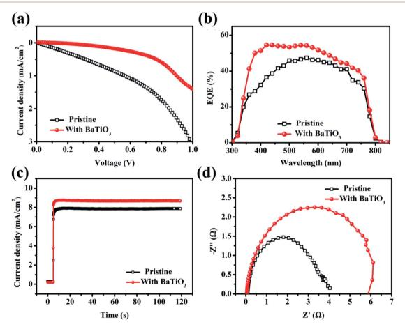
Fig. 5 (a) Dark current curve, (b) EQE curve, and (c) steady-state output current curve at the maximum power point. (d) Impedance diagram of the MAPbl<sub>3</sub> and BaTiO<sub>3</sub>@MAPbl<sub>3</sub>-based C-PSCs.
