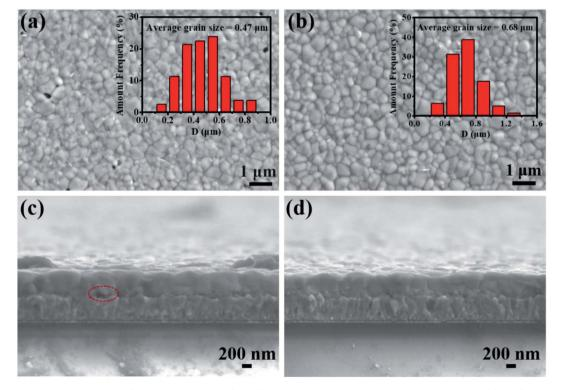
Fig. 3 FE-SEM images of (a)  $FTO/TiO_2/MAPbl_3$  and (b)  $FTO/TiO_2/BaTiO_3:MAPbl_3$ . Cross section images of (c)  $FTO/TiO_2/MAPbl_3$  and (d)  $FTO/TiO_2/BaTiO_3:MAPbl_3$ . The insets in (a) and (b) are the grain size distributions of the corresponding samples.
