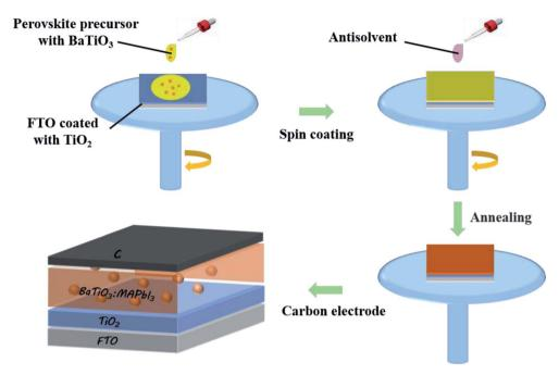
Fig. 1 BaTiO<sub>3</sub>@MAPbl<sub>3</sub> composite film and the device preparation processes.
