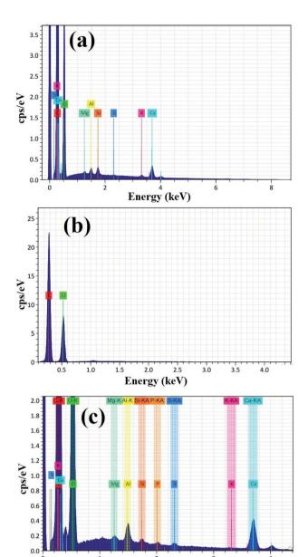
Fig. 4 EDX elemental analysis of (a) pure myrrh, (b) pure PVA, and (c) the PVA/myrrh thin film.
