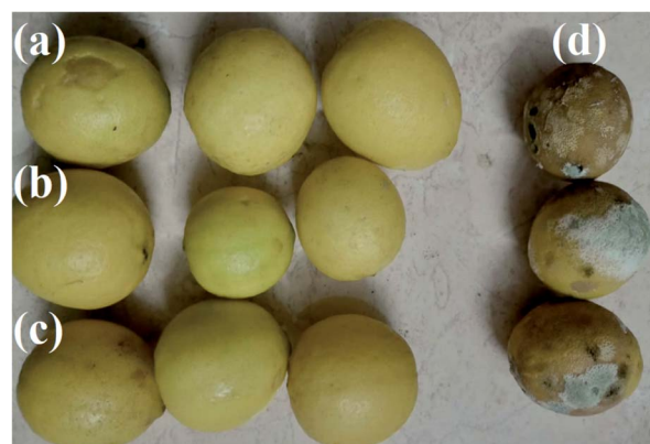
Fig. 7 Effect of the synthesized PVA/myrrh thin film on lemon fruits disease symptoms, where (a) is coated with 1% PVA/myrrh thin film, (b) is coated with 2% PVA/myrrh thin film, (c) is coated with 3% PVA/myrrh thin film, and (d) the untreated control.
