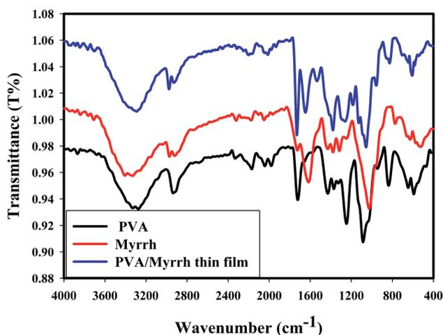
Fig. 2 FTIR analysis of PVA, myrrh natural resin, and the PVA/myrrh thin film.
