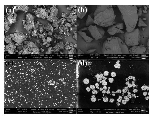
Fig. 3 SEM imaging of (a) pure myrrh, (b) pure PVA, (c) the PVA/myrrh thin film, and (d) magnified image of the synthesized PVA/myrrh thin film.
