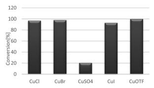
Fig. 3 The catalytic efficiency of various metal (CuI) salts on the aerobic oxidation. Reaction conditions: 1-octanol (1 mmol, 130.2 mg), NMI (0.05 mmol, 8.22 mg), TEMPO (0.05 mmol, 14.8 mg), L4 (0.05 mmol), air, 25  $^{\circ}$ C, 24 h. Conversion calculated by GC analysis using 1,2-dichlorobenzene as internal standard.
