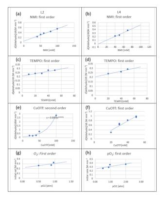
Fig. 5 The kinetic data from oxidation of PhCH $_2$ OH by L/Cu(OTf)/TEMPO assigns the following parameters (a and b) base NMI on L2 and L4, (c and d) TEMPO on L2 and L4, (e and f) CuOTF effect on L2 and L4, and (g and h)  $O_2$  pressure on L2 and L4. Standard reaction conditions: PhCH $_2$ OH (1 mmol, 130.2 mg), Cu(OTf) (0.05 mmol, 18.8 mg), L4 or L4 (0.05 mmol), TEMPO (0.05 mmol, 14.8 mg), air, 25 °C. Conversion calculated by GC analysis using 1,2-dichlorobenzene as internal standard
