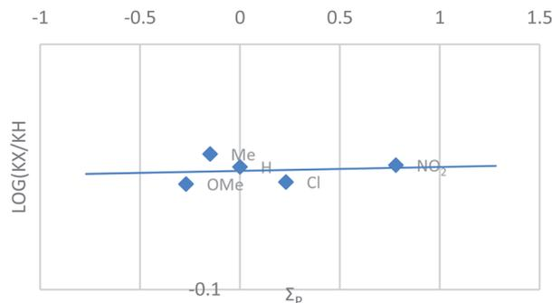
Fig. 7 Hammett plots reflecting a comparison of independent rate measurements of the *para* substituted  $PhCH_2OH$  using L2. Standard reaction conditions:  $PhCH_2OH$  (1 mmol, 130.2 mg),  $Cu(OTf)$  (0.05 mmol, 18.8 mg), L2 (0.05 mmol, 9.2 mg), TEMPO (0.05 mmol, 14.8 mg), air, 25 °C. Conversion calculated by GC analysis using 1,2-dichlorobenzene as internal standard.
