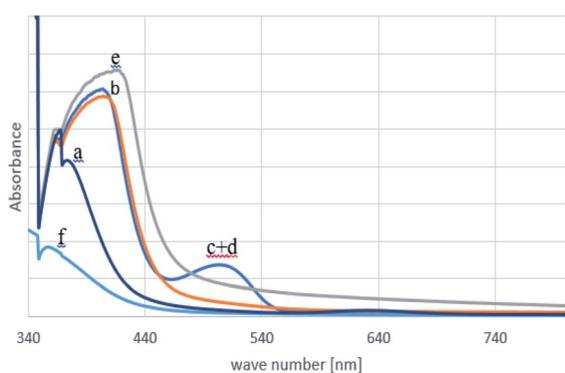
Fig. 6 Subsequent UV-Vis spectra of complex 0.01 mmol  $Cu^I$ OTf/L4 in acetonitrile solution (a) with L4, (b) after 20 min bubbling  $O_2$  through this solution at 20 °C, (c) with NMI after 5 min, (d) with TEMPO immediately, (e) with BzOH immediately, and (f) BzOH 30 min.
