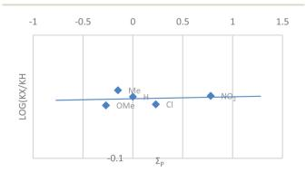
Fig. 7 Hammett plots reflecting a comparison of independent rate measurements of the *para* substituted PhCH<sub>2</sub>OH using L2. Standard reaction conditions: PhCH<sub>2</sub>OH (1 mmol, 130.2 mg), Cu(OTf) (0.05 mmol, 18.8 mg), L2 (0.05 mmol, 9.2 mg), TEMPO (0.05 mmol, 14.8 mg), air, 25 °C. Conversion calculated by GC analysis using 1,2-dichlorobenzene as internal standard.
