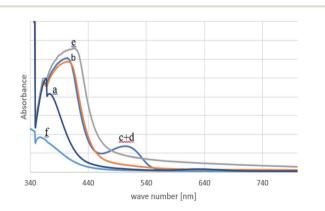
Fig. 6 Subsequent UV-Vis spectra of complex 0.01 mmol Cu<sup>I</sup>OTf/L4 in acetonitrile solution (a) with L4, (b) after 20 min bubbling  $O_2$  through this solution at 20 °C, (c) with NMI after 5 min, (d) with TEMPO immediately, (e) with BzOH immediately, and (f) BzOH 30 min.
