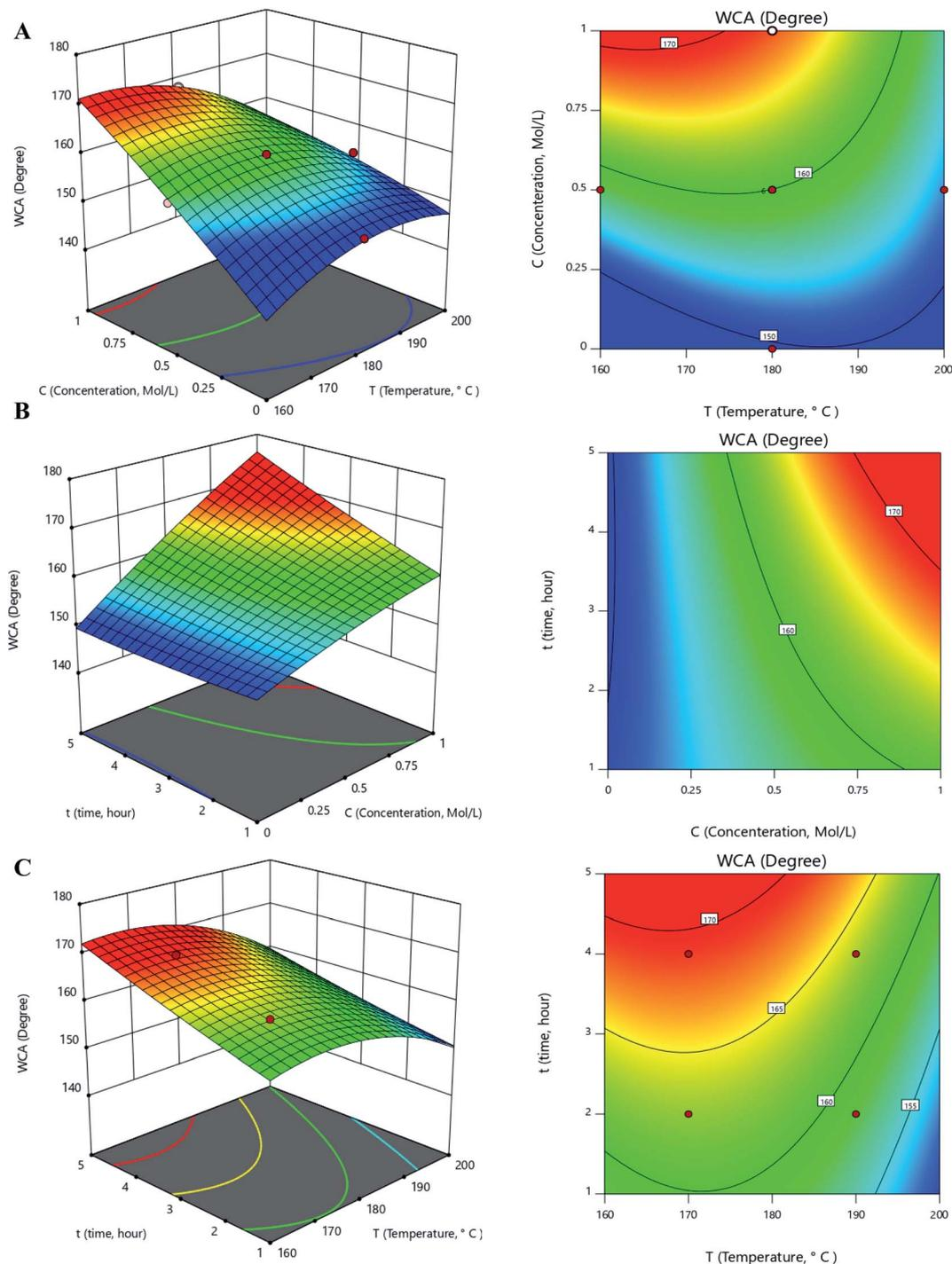
Fig. 5 3D response surface and contour plot of WCA: (A) the interaction between concentration and temperature at a constant time,  $t = 3$  h. (B) The interaction between concentration and time at a constant temperature,  $T = 180$  °C. (C) The interaction between temperature and time at a constant concentration,  $C = 0.5$  Mol/L<sup>-1</sup>.
