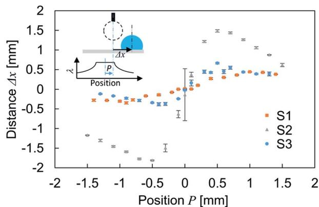
Fig. 4 Relation between droplet deposition position  $P$  and transfer distance  $\Delta x$ . The error bars show the standard deviation. The inset schematics show the experimental details. The bottom graph illustrates the relation between position and structural wavelength.
