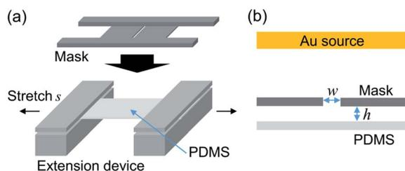
Fig. 1 (a) Schematics of the extension device. (b) Illustration of the deposition region. The slit width of the installed mask and distance between the mask and PDMS surface are  $w$  and  $h$ , respectively.
