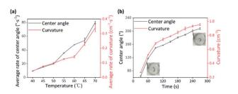
Fig. 5 (a) Average rate of the two parameters; (b) center angles and curvature change of bilayer hydrogel in solution with a higher concentration of SDS (1.5 mg  $\rm mL^{-1}$ ).
