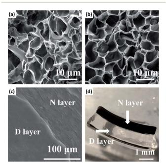
Fig. 2 SEM images of (a) D layer, (b) N layer and (c) the interface; (d) photo of the prepared bilayer hydrogel cut in a size of 4.2 mm  $\times$  2.2 mm  $\times$  1.3 mm.
