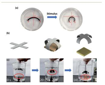
Fig. 8 (a) Bending behavior of the bilayer hydrogel and reference system; schematic illustration (b) and digital images (c) of the gripping and release using the 4-arm gripper (the copper sheet is marked by the red circle).
