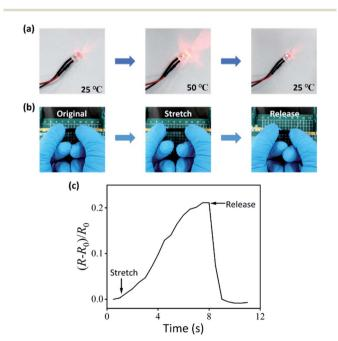
Fig. 9 (a) Brightness changes of the LED when the bilayer hydrogel was immersed in deionized water in the order of  $25\,^{\circ}\text{C}-50\,^{\circ}\text{C}-25\,^{\circ}\text{C}$ . The correlation between (b) stretching degree and (c) resistance change rate of the bilayer hydrogel.
