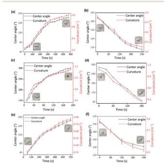
Fig. 6 The center angles and curvatures of bilayer hydrogel in solutions of 1 M HCl (a), 1 M NaOH (c), 1 M NaCl (e) and their respective recovery (b), (d), (f).
