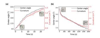
Fig. 4 Center angles and curvatures of the bilayer hydrogel at 40  $^{\circ}$ C (a) and its recovery (b).
