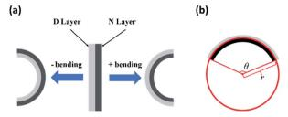
Fig. 3 (a) Positive and negative bending directions; (b) simplified model for calculating the center angle and curvature of the bent hydrogel ( $\theta$  is the center angle corresponding to the arc, and r is the radius of the circle)
