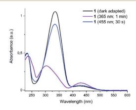
Fig. 3 UV-vis spectra of the compound 1 in darkness, after irradiation with UV (365 nm) and with blue (455 nm) light. The curves after irradiation correspond to the photostationary states and distinct isosbestic points are displayed.
