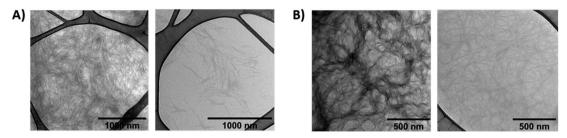
Fig. 7 Transmission electron microscopy (TEM) of the hydrogels (without additional staining). (A) gel A (1.5 wt% of 1 in PBS pH 7.4) – dark-adapted (left) and irradiated with 365 nm UV light (right); (B) gel B (0.6 wt% of 1 + 0.6 wt% of alginate in diH<sub>2</sub>O) – dark-adapted (left) and irradiated with 365 nm UV light (right).
