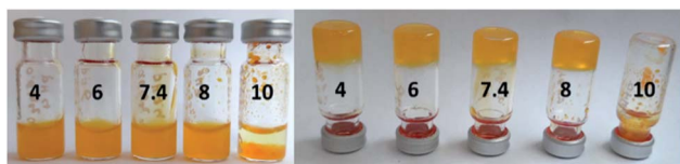
Fig. 9 The hydrogels composed of 0.6 wt% 1 and 0.6 wt% of alginate in buffers. The respective pH values (in the range pH 4–pH 10) are indicated.
