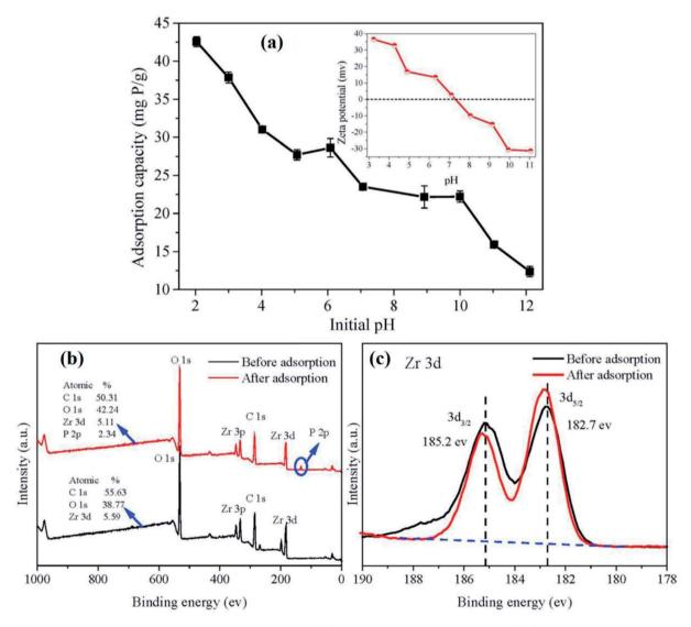
Fig. 12 (a) Effect of pH on the adsorption of phosphate on Zr-GO/Alq aerogel beads and XPS of Zr-GO/Alq before and after the adsorption process. (b) Wide spectra and (c) Zr 3d spectra. This figure reproduced from ref. 128 with permission from Elsevier. Copyright (2019).
