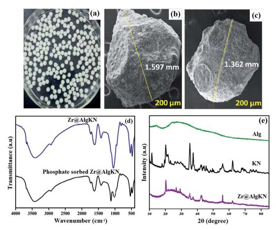
Fig. 5 (a) Digital image for Zr@AlgKN, (b) SEM of Zr@AlgKN (in situ), (c) SEM of Zr@AlgKN (hydro), (d) FTIR spectra of Zr@AlgKN before and after the adsorption of phosphate, and (e) XRD patterns of Alg, KN and Zr@AlgKN. This figure reproduced from ref. 85 with permission from Elsevier. Copyright (2020).
