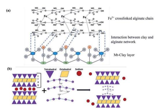
Fig. 4 (a) The crosslinking process of Fe<sup>3+</sup> to Alg network and interaction with Mt and (b) the possible MtlAlg network configuration. This figure reproduced from ref. 82 with permission from Elsevier. Copyright (2021).
