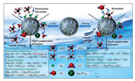
Fig. 7 The multiple forms of phosphate ions and the possible mechanism to adsorb phosphate ions onto Alg-Mgo@BT. This figure reproduced from ref. 90 with permission from Elsevier. Copyright (2021).
