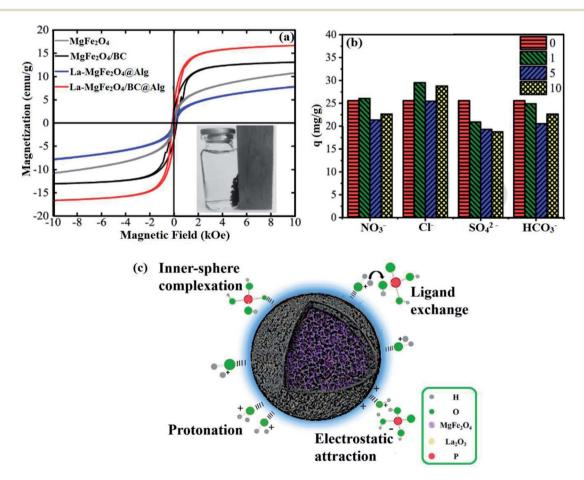
Fig. 9 (a) VSM measurement, (b) effect of different concentrations of coexisting ions on phosphate adsorption, and (c) the proposed adsorption mechanisms of phosphate onto La-MgFe<sub>2</sub>O<sub>4</sub>/BC@Alg. This figure reproduced from ref. 100 with permission from Elsevier. Copyright (2021).
