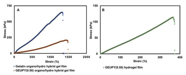
Fig. 7 Stress strain curve for (A) gelatin organo/hydro hybrid gel films, GEUPY(0.50) organo/hydro hybrid gel films and (B) GEUPY(0.50) hydrogel films.
