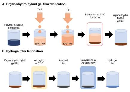
Fig. 5 Schematics to demonstrate the fabrication of (A) organo/hydro hybrid gel films and (B) hydrogel films.
