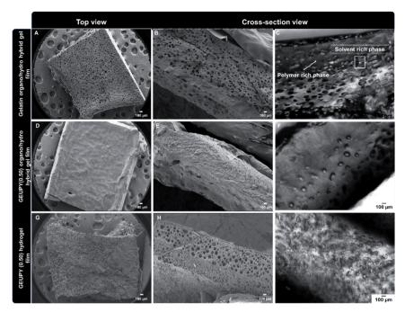
Fig. 6 SEM images of freeze dried gelatin (A–C), GEUPY(0.50) organo/hydro hybrid gel films (D–F) and rehydrated GEYPY(0.050) hydrogel films (G–I). Top view (A, D and G), cross-section view (B, E, and H) and optical microscopic images of respective films cross-section (C, F, and I).
