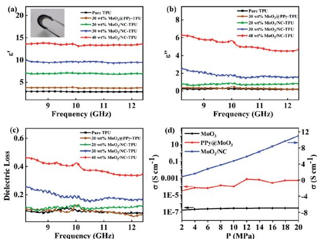
Fig. 6 Frequency dependence on (a) real, (b) imaginary part of the complex permittivity and (c) dielectric loss in X band, (d) the powder electric conductivity of different samples within 2–20 MPa.
