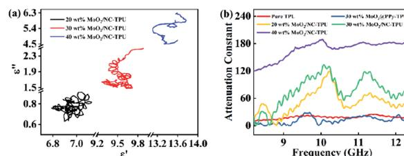
Fig. 7 (a) The  $\epsilon' - \epsilon''$  curves of MoO<sub>2</sub>/NC-TPU composites under different filler loadings; (b) attenuation constants of various samples.
