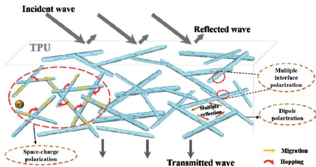
Fig. 8 The possible wave absorption mechanism of MoO<sub>2</sub>/NC-TPU composites.
