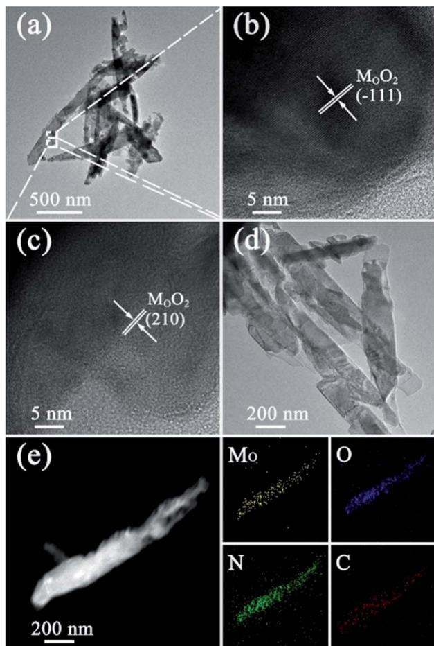
Fig. 4 (a and d) TEM images, (b and c) HRTEM images of MoO<sub>2</sub>/NC heteronanowires; (e) the elemental mappings of Mo, O, N and C.
