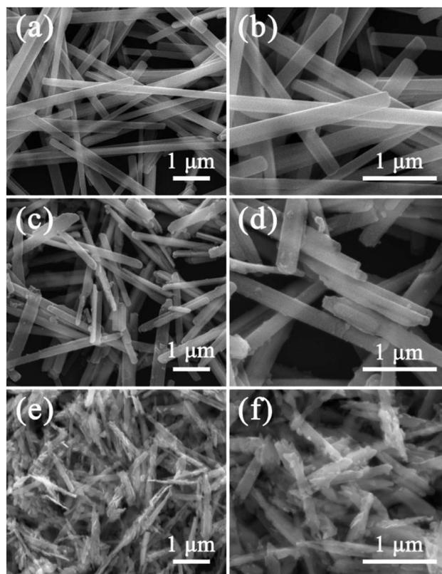
Fig. 3 SEM images of (a and b) MoO<sub>3</sub> nanowires; (c and d) MoO<sub>3</sub>@PPy nanowires and (e and f) MoO<sub>2</sub>/NC heteronanowires.
