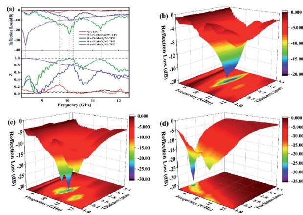
Fig. 5 (a) Microwave RL curves of the samples with a thickness of 2.3 mm in X band. Three-dimensional representations of the RL of MoO<sub>2</sub>/NC-TPU composites with a loading of (b) 20 wt%, (c) 30 wt% and (d) 40 wt%.
