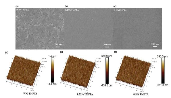
Fig. 3 (a-c) Top-view SEM images and (d-f) 3D topographical AFM images of the quasi-2D perovskite films without or with TMPTA modification.
