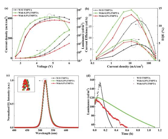
Fig. 2 (a) Current density-voltage-luminance (J-V-L) curves, (b) current efficiency and external quantum efficiency versus current density (CE-J and EQE-J) curves, (c) normalized EL spectra, and (d) device degradation profiles aged under a constant current enabling an initial luminance of 100 cd m<sup>-2</sup> of the PeLEDs without and with TMPTA modification. The ratio of TMPTA is its concentration in antisolvent.
