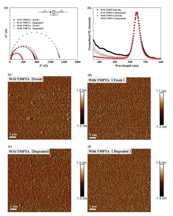
Fig. 7 (a) EIS spectra of the PeLEDs without and with TMPTA modification before and after aging. (b) PL spectra and (c-f) AFM images of the perovskite films obtained from the fresh and degraded PeLEDs. The perovskite films were obtained by peeling off the metal cathode and washing away the organic electron transport materials.
