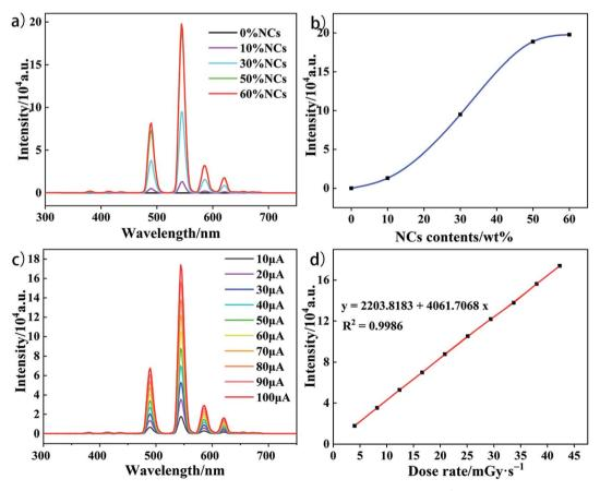
Fig. 5 (a) RL intensity of the composite films with different NCs contents (wt%) under 42.29 mGy s<sup>-1</sup> X-ray irradiation. (b) Variation curve of RL peak intensity at 544 nm with different loading rate. (c) RL spectrum of 50 wt% NCs loaded composite film under 50 keV tube voltage and different tube currents (10–100 μA). (d) RL intensity at 544 nm of 50 wt% NCs loaded composite film under different dose rate X-ray irradiation.
