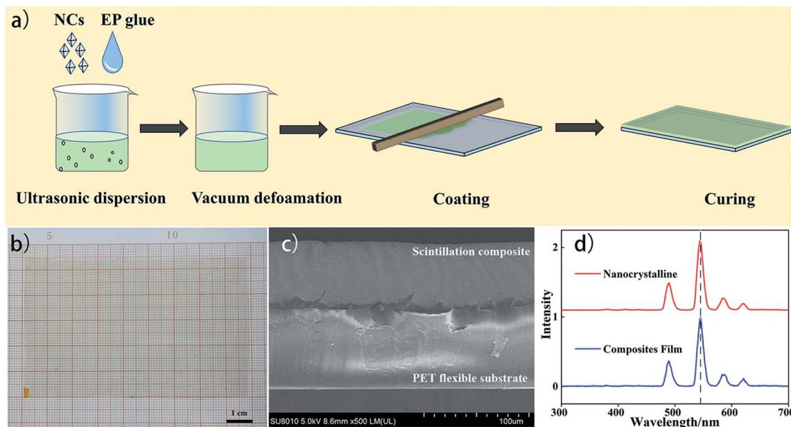
Fig. 4 (a) Schematic diagram of preparation process of  $\text{LiLuF}_4:15\% \text{Tb}$  NCs-EP composite scintillating film. (b) The photograph of composite film with 50 wt% NCs loading. (c) The cross section SEM image of composite film with 50 wt% NCs loading. (d) RL spectrum of  $\text{LiLuF}_4:\text{Tb}$  NCs and composite films.
