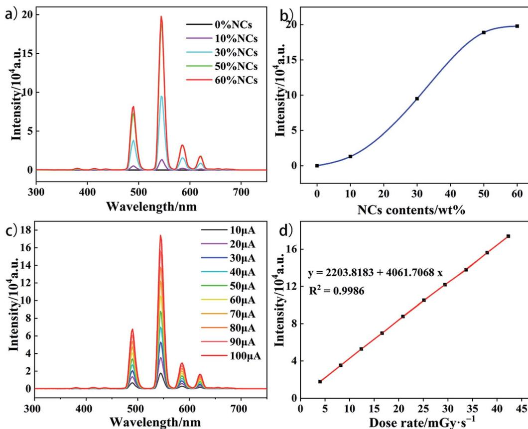
Fig. 5 (a) RL intensity of the composite films with different NCs contents (wt%) under  $42.29 \text{ mGy s}^{-1}$  X-ray irradiation. (b) Variation curve of RL peak intensity at 544 nm with different loading rate. (c) RL spectrum of 50 wt% NCs loaded composite film under 50 keV tube voltage and different tube currents (10–100  $\mu\text{A}$ ). (d) RL intensity at 544 nm of 50 wt% NCs loaded composite film under different dose rate X-ray irradiation.
