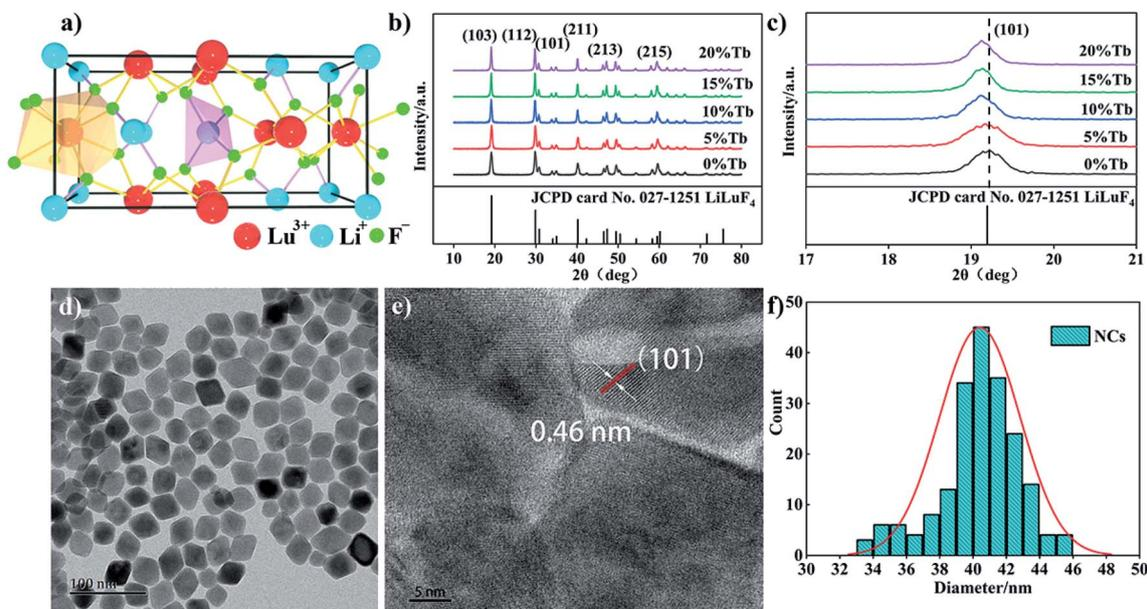
Fig. 1 (a) Crystal structure diagram of LiLuF<sub>4</sub>. (b) X-ray diffraction patterns of LiLuF<sub>4</sub>:xTb (*x* = 0%, 5%, 10%, 15% and 20%) NCs. (c) The X-ray diffraction peaks of (101) facets of LiLuF<sub>4</sub>:xTb (*x* = 0%, 5%, 10%, 15% and 20%) NCs. (d) The transmission electron microscope image of LiLuF<sub>4</sub>:15%Tb NCs. (e) The high-resolution TEM of a single LiLuF<sub>4</sub>:15%Tb NCs. (f) Statistics graph of nanocrystalline particle size distribution.
