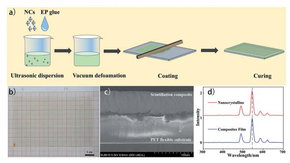
Fig. 4 (a) Schematic diagram of preparation process of  $LiLuF_4$ : 15% Tb NCs-EP composite scintillating film. (b) The photograph of composite film with 50 wt% NCs loading. (c) The cross section SEM image of composite film with 50 wt% NCs loading. (d) RL spectrum of  $LiLuF_4$ : Tb NCs and composite films.
