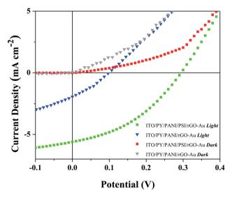
Fig. 2 J-V plots of BPV cells with and without PSI in dark and under simulated sunlight with an intensity of 1000 W m<sup>-2</sup>.
