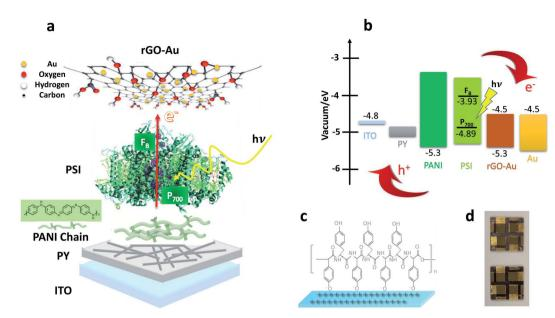
Fig. 1 (a) Solid-state PSI-based photovoltaic cell with labeled components. (b) Energy levels of each layer and charge transfer pathways to external electrodes of biophotovoltaic cell. (c) Assembly of polytyrosine on positive ITO surface. (d) A photograph of completed BPV devices (the energy level data are given elsewhere. <sup>23,53-57</sup>).
