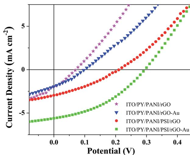
Fig. 3  $J$ - $V$  curves of four different photovoltaic cells fabricated with rGO-Au and rGO layer in the presence and absence of PSI under AM1.5G illumination. BPV cells fabricated of ITO/PY/PANI/PSI/rGO-Au (green), ITO/PY/PANI/PSI/rGO (blue), ITO/PY/PANI/rGO-Au (orange), and ITO/PY/PANI/rGO (magenta).
