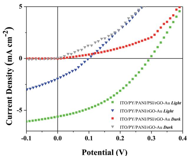
Fig. 2  $J$ - $V$  plots of BPV cells with and without PSI in dark and under simulated sunlight with an intensity of  $1000 \text{ W m}^{-2}$ .
