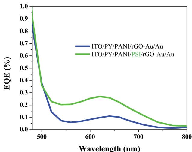
**Fig. 4** External quantum efficiency (EQE) of fabricated BPV cells with and without PSI as active layer between PANI and rGO–Au charge transfer layers.
