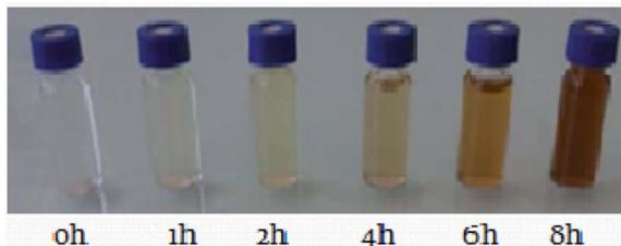
Fig. 1 Intensity evolution of color aqueous solution during Tyr conversion over time:  $[Tyr] = 10^{-2}$  M;  $[H_2O_2] = 5.05 \times 10^{-3}$  M, KSF =  $0.2$  g L<sup>-1</sup>.
