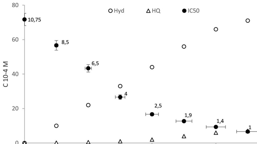
Fig. 8 Free radical scavenging activity during catalytic oxidation of Tyr over the following conditions:  $10^{-2}$  M [Tyr],  $7 \times 10^{-2}$  M [ $\text{H}_2\text{O}_2$ ] and  $0.2 \text{ g L}^{-1}$  [KSF].
