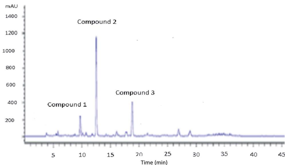
Fig. 2 HPLC chromatogram of Tyr oxidation after 4 hours. Peaks: compound 1: HQ; compound 2: Hyd; compound 3: Tyr. Experiment conditions:  $[Tyr] = 10^{-2}$  M;  $[H_2O_2] = 5.05 \times 10^{-3}$  M, KSF =  $0.2$  g L<sup>-1</sup>.
