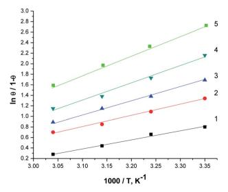
Fig. 10 The relationship between  $\log (\theta/1 - \theta)$  versus 1/T for X80 CS in 0.5 M H<sub>2</sub>SO<sub>4</sub> containing different doses of parsley oil. (1) 50 ppm parsley oil (2) 150 ppm (3) 250 ppm (4) 350 ppm (5) 450 ppm.
