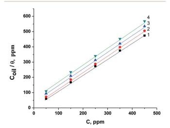
Fig. 9 Langmuir isotherm relationship for the corrosion of X80 CS in  $0.5 \text{ M} \text{ H}_2\text{SO}_4$  including some doses of parsley oil at certain temperatures. (1) 298 K (2) 308 K (3) 318 K (4) 328 K.
