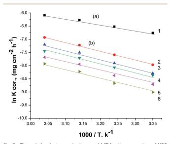
Fig. 7 The relation between  $\ln K_{\rm corr}$  and 1/T for the corrosion of X80 CS in 0.5 M  $\rm H_2SO_4$  including some doses of parsley oil [a] (1) 0.5 M  $\rm H_2SO_4$ . [b] (2) 50 ppm (3) 150 ppm (4) 250 ppm (5) 350 ppm (6) 450 ppm.
