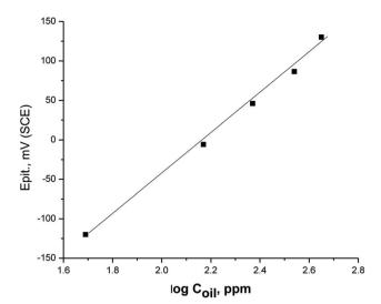
Fig. 5 A plot between  $E_{\rm pit}$  and log  $C_{\rm oit}$  for X80 CS in 0.5 M H<sub>2</sub>SO<sub>4</sub> + 0.5 M NaCl solutions\_+ different doses of parsley oil.
