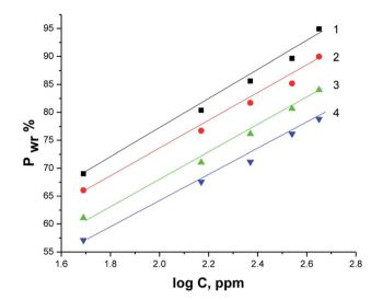
Fig. 6 The relationship between  $P_{\rm wr}$ % and log  $C_{\rm oil}$  for X80 CS in 0.5 M  $H_2{\rm SO}_4$  containing different doses of parsley oil at different temperatures. (1) 298 K (2) 308 K (3) 318 K (4) 328 K.
