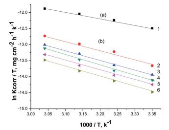
Fig. 8 The relation between  $\ln K_{corr}/T$  and 1/T for the corrosion of X80 CS in 0.5 M  $H_2SO_4$  including some doses of parsley oil [a] (1) 0.5 M  $H_2SO_4$ . [b] (2) 50 ppm (3) 150 ppm (4) 250 ppm (5) 350 ppm (6) 450 ppm.
