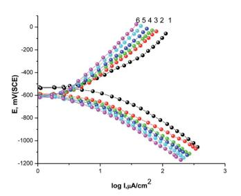
Fig. 1 GAP curves of X80 CS in 0.5 M H<sub>2</sub>SO<sub>4</sub> as well as containing certain concentricity of parsley oil. (1) 0.00 (2) 50 (3) 150 (4) 250 (5) 350 (6) 450 ppm.
