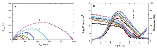
Fig. 2 Nyquist (a) and Bode plots (b) of X80 CS corrosion in 0.5 M H<sub>2</sub>SO<sub>4</sub> alone and in the presence of certain concentrations of parsley oil at 298 K. (1) 0.00 (2) 50 (3) 150 (4) 250 (5) 350 (6) 450 ppm.
