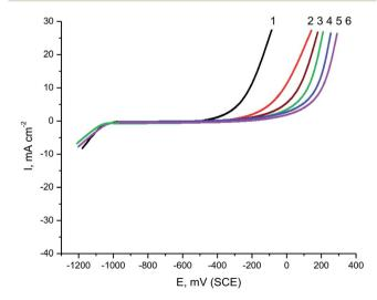
Fig. 4 PDAP curves of X80 CS in  $0.5 \text{ M} \text{ H}_2\text{SO}_4 + 0.5 \text{ M}$  NaCl solutions containing different concentrations of parsley oil. (1) 0.00 (2) 50 (3) 150 (4) 250 (5) 350 (6) 450 ppm.
