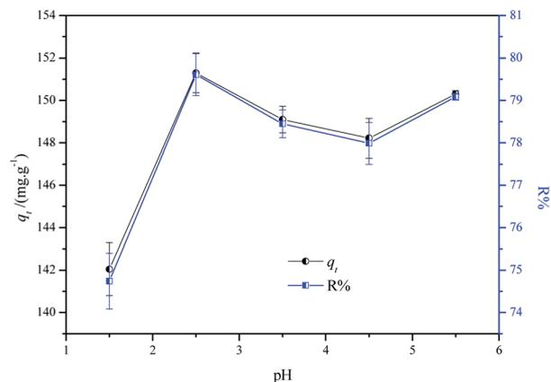
Fig. 6 Effect of pH on the adsorption process (experimental conditions: adsorbent dosage,  $1.6 \text{ g L}^{-1}$ ; initial concentration,  $300 \text{ mg L}^{-1}$ ; temperature,  $30 \text{ }^\circ\text{C}$ ; contact time, 2 h; pH = 1.5, 2.5, 3.5, 4.5, and 5.5).
