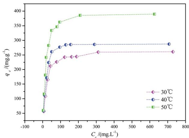
Fig. 11 Adsorption isotherms for Isolan Black 2S-LD at an initial dye concentration between 50 mg L<sup>-1</sup> and 1000 mg L<sup>-1</sup>, an adsorption dosage of 0.5 g L<sup>-1</sup>, and temperatures of 30 °C, 40 °C, and 50 °C.
