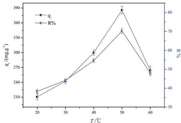
Fig. 8 Effect of reaction temperature on the adsorption process (experimental conditions: adsorbent dosage = 2 g L<sup>-1</sup>, initial concentration = 1000 mg L<sup>-1</sup>, temperature = 20, 30, 40, 50, and 60 °C, contact time = 2 h, and initial pH 3.0).
