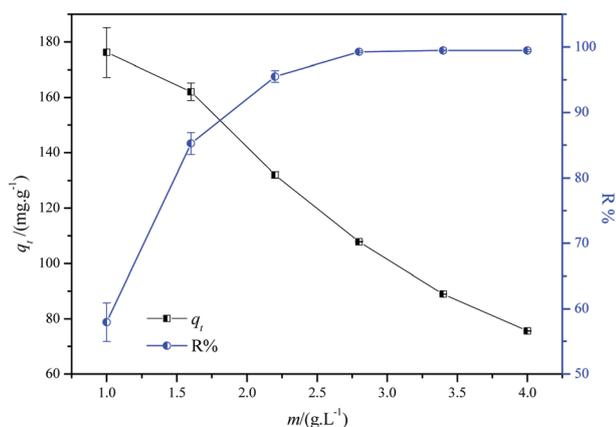
Fig. 7 Effect of adsorbent dosage on the adsorption process (experimental conditions: adsorbent dosage = 1, 1.6, 2.2, 2.8, 3.4, and 4 g L<sup>-1</sup>, initial concentration = 300 mg L<sup>-1</sup>, temperature = 30 °C, contact time = 2 h, initial pH = 3.0, and volume of dye solution = 50 mL).
