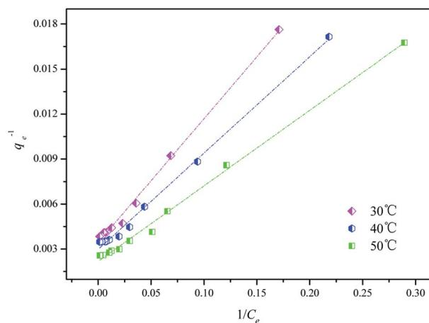
Fig. 12 Langmuir isotherms for Isolan Black 2S-LD at an initial dye concentration between 50 mg L<sup>-1</sup> and 1000 mg L<sup>-1</sup>, an adsorption dosage of 0.5 g L<sup>-1</sup>, and temperatures of 30 °C, 40 °C, and 50 °C.
