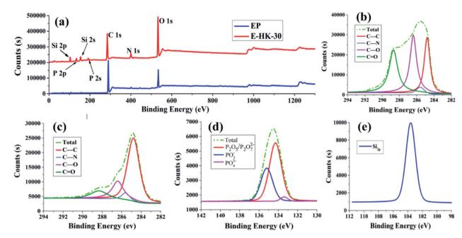
Fig. 4 Structural characterization of CR-EP and CR-E-HK-30. (a) XPS of CR-EP and CR-E-HK-30; (b) C 1s spectra of CR-EP; (c) C 1s spectra of CR-E-HK-30; (d) P 2p spectra of CR-E-HK-30; (e) Si 2p spectra of CR-E-HK-30, respectively.
