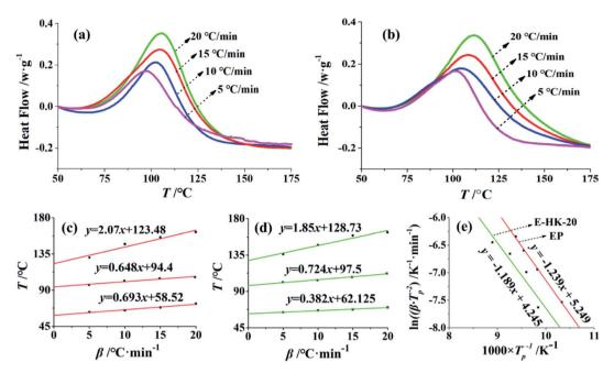
Fig. 2 DSC thermograms of EP (a) and E-HK-20 (b),  $T-\beta$  curve of EP (c) and E-HK-20 (d) at different  $\beta$  under N<sub>2</sub> atmosphere, and  $\ln(\beta/T_p^2)-1/T_p$  curve by Kissinger method in different curing reaction (e).
