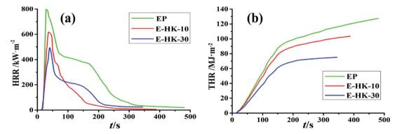
Fig. 6 HRR curves (a) and THR curves (b) for samples under an external heat flux of 50 kW m<sup>-2</sup>.
