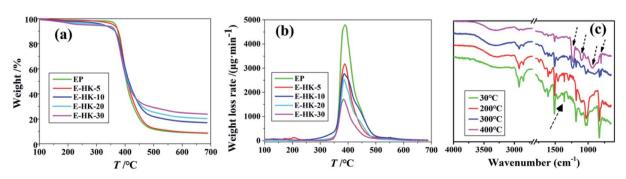
Fig. 3 Thermal stability of EP and E-HK: (a) TG curves, and (b) weight loss rate (c) FTIR spectra of E-HK composites at different temperatures.
