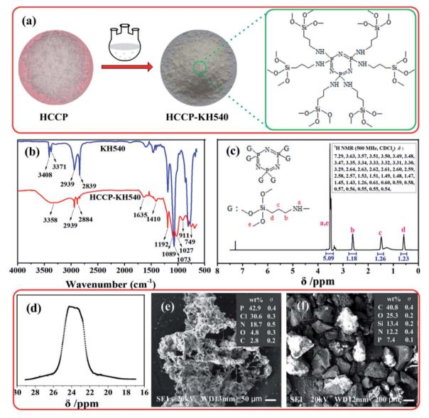
Fig. 1 Synthesis route, element and structure analysis of HCCP-KH540: (a) synthesis route; (b) FTIR of HCCP and HCCP-KH540; (c) <sup>1</sup>H NMR of HCCP-KH540; (d) <sup>31</sup>P NMR of HCCP-KH540; (e and f) SEM of HCCP and HCCP-KH540, the inset shows element content measurement result by EDS.
