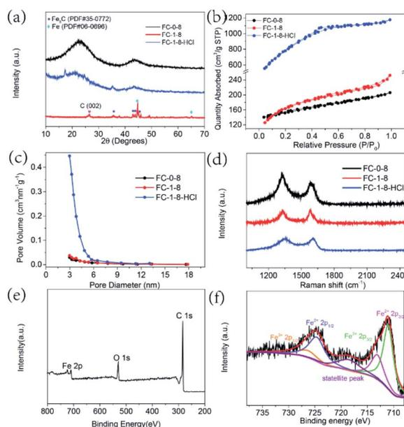
Fig. 2 (a–d) XRD, N<sub>2</sub> adsorption–desorption isotherms, pore size distribution curves and Raman spectra of FC-0-8, FC-1-8 and FC-1-8-HCl. (e and f) XPS spectra of survey and high-resolution Fe 2p of FC-1-8 sample.
