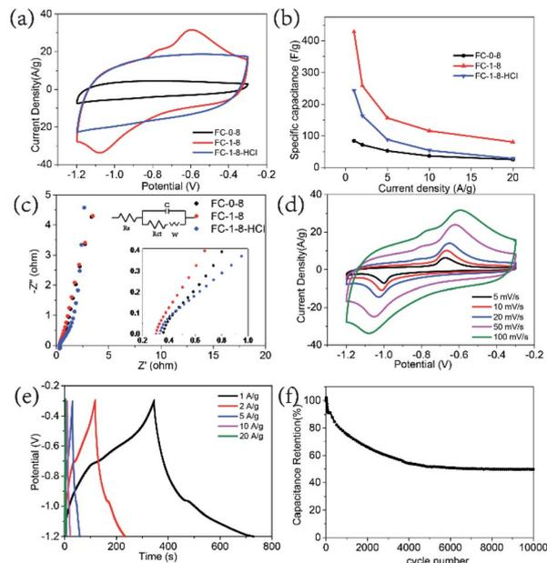
Fig. 5 (a) CV curves at a scan rate of 100  $\text{mV s}^{-1}$  of FC-0-8, FC-1-8 and FC-1-8-HCl, respectively. (b) Rate capability at a current density from 1 to 20  $\text{A g}^{-1}$  and (c) EIS of the samples. (d and e) CV curves and galvanostatic charge–discharge curves of FC-1-8. (f) Cycling performance of FC-1-8 at 5  $\text{A g}^{-1}$  for 10 000 cycles.
