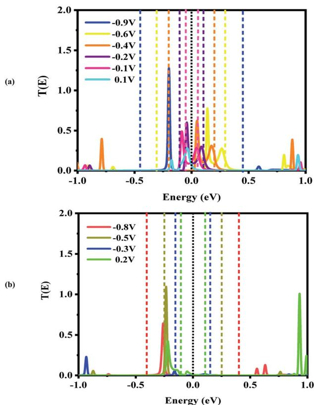
Fig. 6 Bias-dependent transmission spectra of the CNT|C-(B-C)<sub>2</sub>-C|CNT molecular device at different voltages, (a) -0.9, -0.6, -0.4, -0.2, -0.1 and 0.1 V and (b) -0.8, -0.5, -0.3 and 0.2 V. The Fermi level (black dotted line) is set to zero and the energy region between the two dashed lines shows the bias window.
