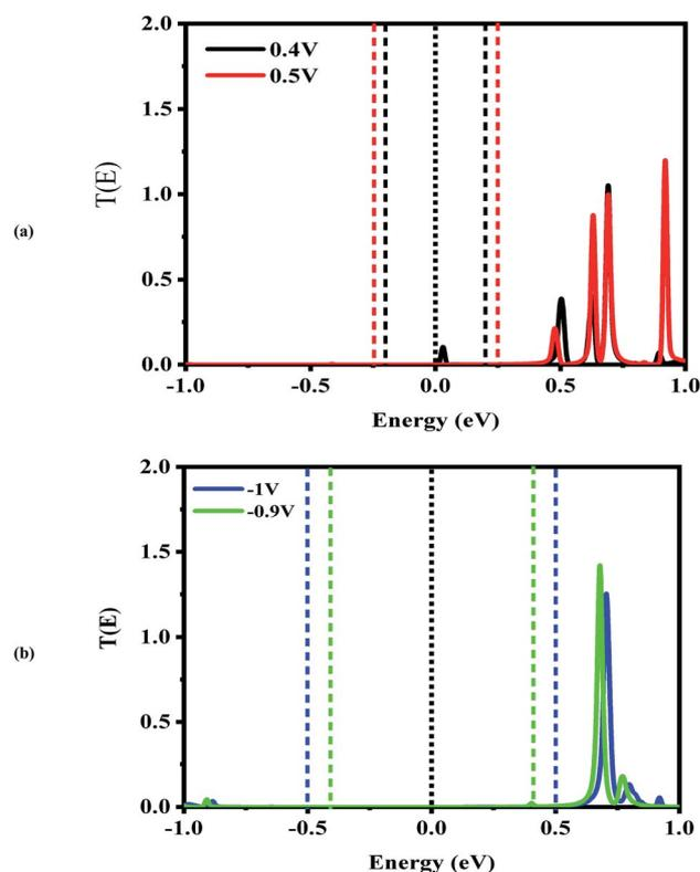
Fig. 5 Bias-dependent transmission spectra of the CNT|C-(Si-C)<sub>2</sub>-C|CNT molecular device at different voltages, (a) 0.4 and 0.5 V and (b) -0.9 and -1.0 V. The Fermi level (black dotted line) is set to zero and the energy region between the two dashed lines shows the bias window.
