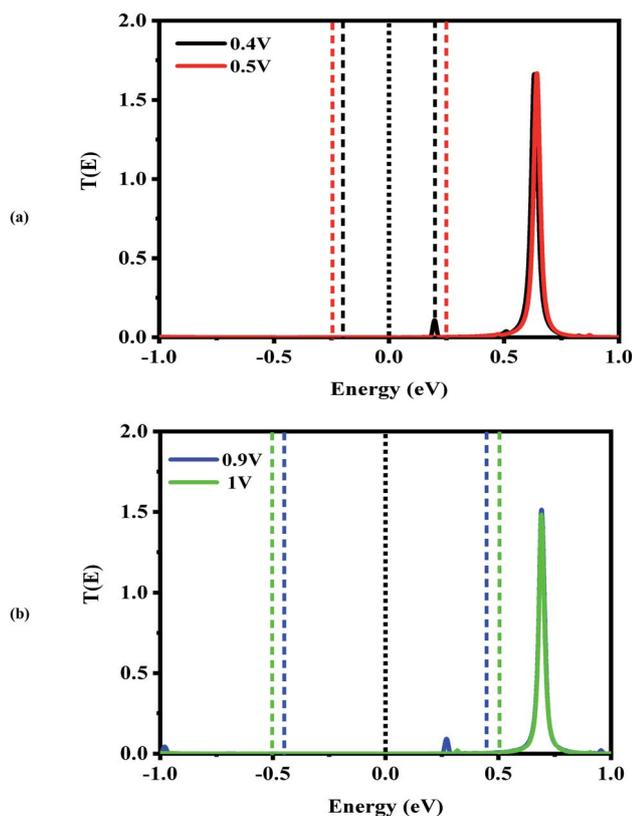
Fig. 4 Bias-dependent transmission spectra of the CNT|C<sub>6</sub>|CNT molecular device at different voltages, (a) 0.4 and 0.5 V and (b) 0.9 and 1.0 V. The Fermi level (black dotted line) is set to zero and the energy region between the two dashed lines shows the bias window.
