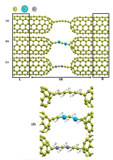
Fig. 1 Final relaxed geometries of (a)  $C_6$ , (b)  $C_7$ C and (c)  $C_7$ C and (c)  $C_7$ C junctions with CNTs electrodes. The number of atoms in each chain is 6. The labels L, SR and R denote the left electrode, the scattering region, and the right electrode, respectively. In (d), the  $C_7$ C, Si- $C_7$ C and B- $C_7$ C bond lengths (Å) in each chain are represented.
