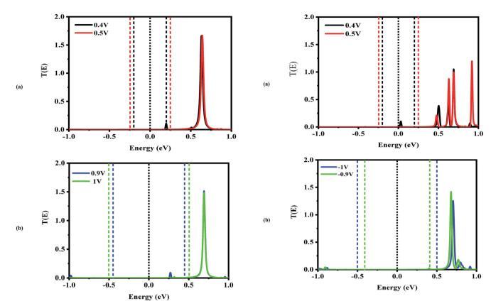
Fig. 4 Bias-dependent transmission spectra of the CNT $|C_6|$ CNT molecular device at different voltages, (a) 0.4 and 0.5 V and (b) 0.9 and 1.0 V. The Fermi level (black dotted line) is set to zero and the energy region between the two dashed lines shows the bias window.
