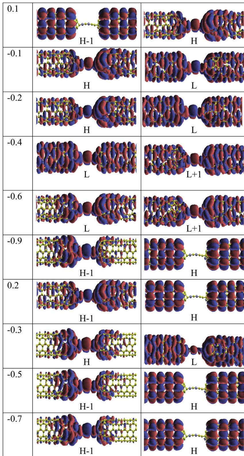
Fig. 7 Frontier molecular distributions of CNT|C-(B-C)<sub>2</sub>-C|CNT device at various bias voltages.
