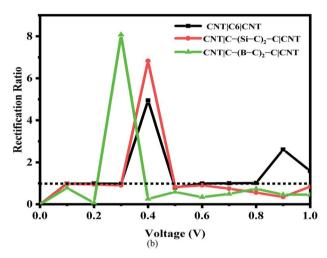
Fig. 2 (a) The I-V curves and (b) rectification ratio change with various bias voltages of  $C_6$ ,  $C-(Si-C)_2-C$  and  $C-(B-C)_2-C$  junctions.  $P_i$  and  $V_i$  (i=1, 2, 3, 4) indicate the peak and valley positions for each junction. The dotted line indicates R(V)=1.
