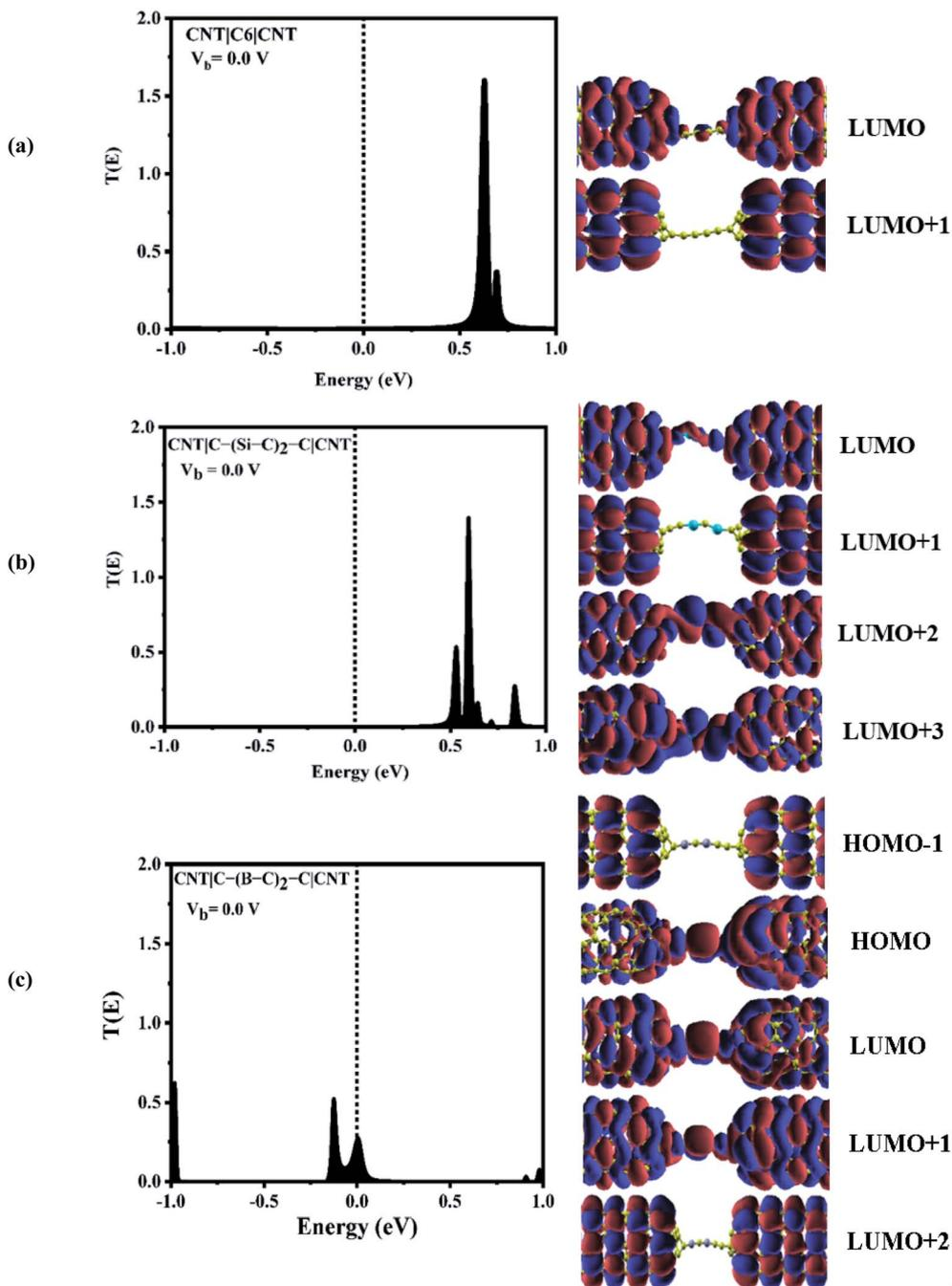
Fig. 3 Left: transmission spectra and spatial distribution of orbitals for (a) CNT|C<sub>6</sub>|CNT, (b) CNT|C-(Si-C)<sub>2</sub>-C|CNT, and (c) CNT|C-(B-C)<sub>2</sub>-C|CNT molecular devices at zero bias. The dashed lines represent the Fermi level. Right: frontier molecular orbitals.
