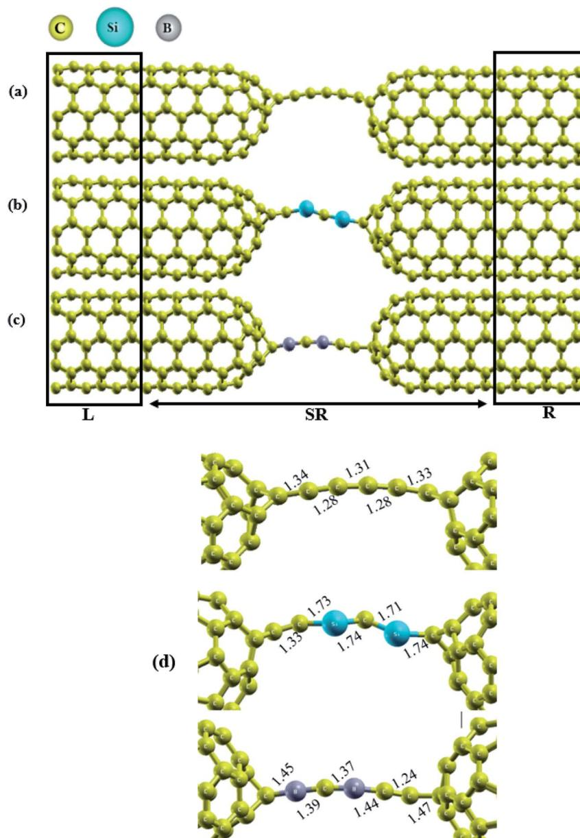
Fig. 1 Final relaxed geometries of (a) C<sub>6</sub>, (b) C-(Si-C)<sub>2</sub>-C and (c) C-(B-C)<sub>2</sub>-C junctions with CNTs electrodes. The number of atoms in each chain is 6. The labels L, SR and R denote the left electrode, the scattering region, and the right electrode, respectively. In (d), the C-C, Si-C and B-C bond lengths (Å) in each chain are represented.
