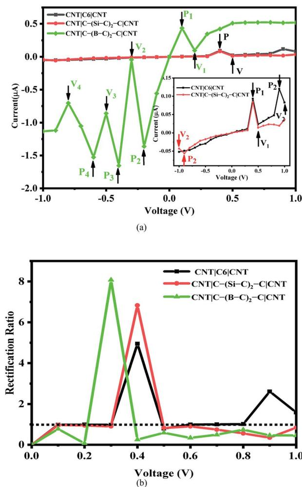
Fig. 2 (a) The  $I$ - $V$  curves and (b) rectification ratio change with various bias voltages of  $C_6$ ,  $C-(Si-C)_2-C$  and  $C-(B-C)_2-C$  junctions.  $P_i$  and  $V_i$  ( $i=1, 2, 3, 4$ ) indicate the peak and valley positions for each junction. The dotted line indicates  $R(V) = 1$ .
