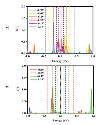
Fig. 6 Bias-dependent transmission spectra of the CNT $|C-(B-C)_2-C|CNT$  molecular device at different voltages, (a) -0.9, -0.6, -0.4, -0.2, -0.1 and 0.1 V and (b) -0.8, -0.5, -0.3 and 0.2 V. The Fermi level (black dotted line) is set to zero and the energy region between the two dashed lines shows the bias window.
