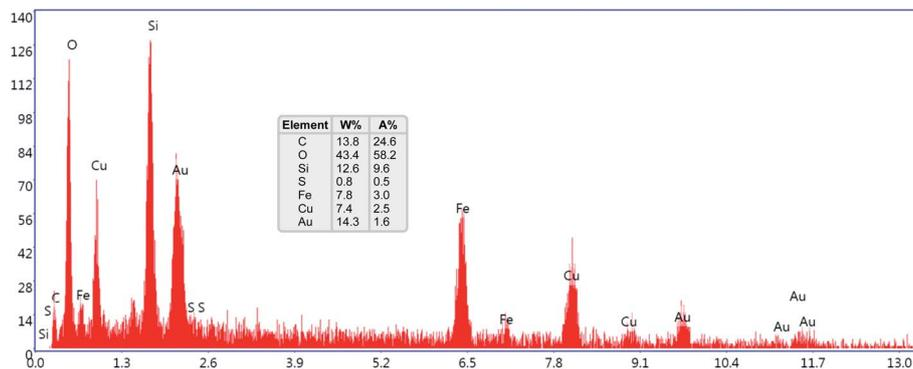
Fig. 6 SEM-based EDX spectrum of the  $\text{Fe}_3\text{O}_4@\text{SiO}_2@\text{KCC-1}@MPTMS@Cu^{II}$  nanocomposite.
