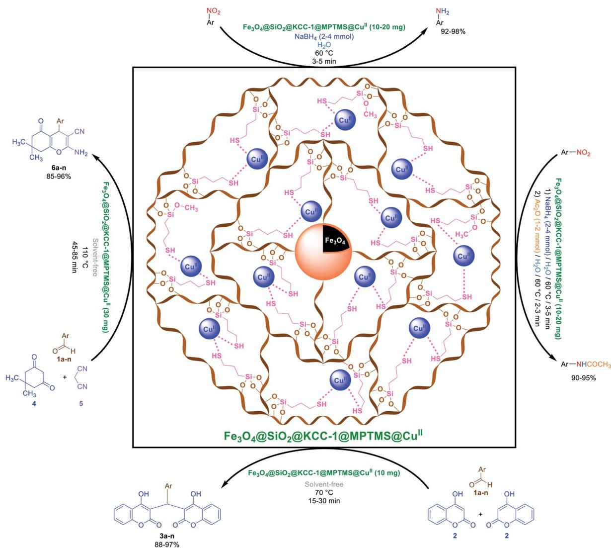
Fig. 1 Catalytic applications of the cockscomb flower-like  $\text{Fe}_3\text{O}_4@SiO_2@KCC-1@MPTMS@Cu^{II}$  mesoporous nanocomposite in the reduction and reductive acetylation of nitroarenes in water and solvent-free one-pot synthesis of some coumarin compounds.
