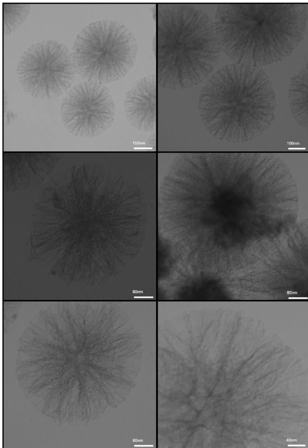
Fig. 5 TEM images of the dendritic  $\text{Fe}_3\text{O}_4@SiO_2@KCC-1@MPTMS@Cu^{II}$  nanocomposite.
