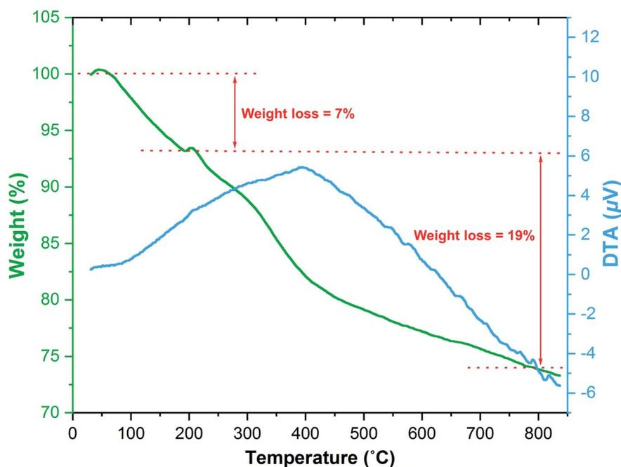
Fig. 7 TGA/DTA diagram of the  $\text{Fe}_3\text{O}_4@\text{SiO}_2@\text{KCC-1}@\text{MPTMS}@\text{Cu}^{\text{II}}$  nanocomposite.
