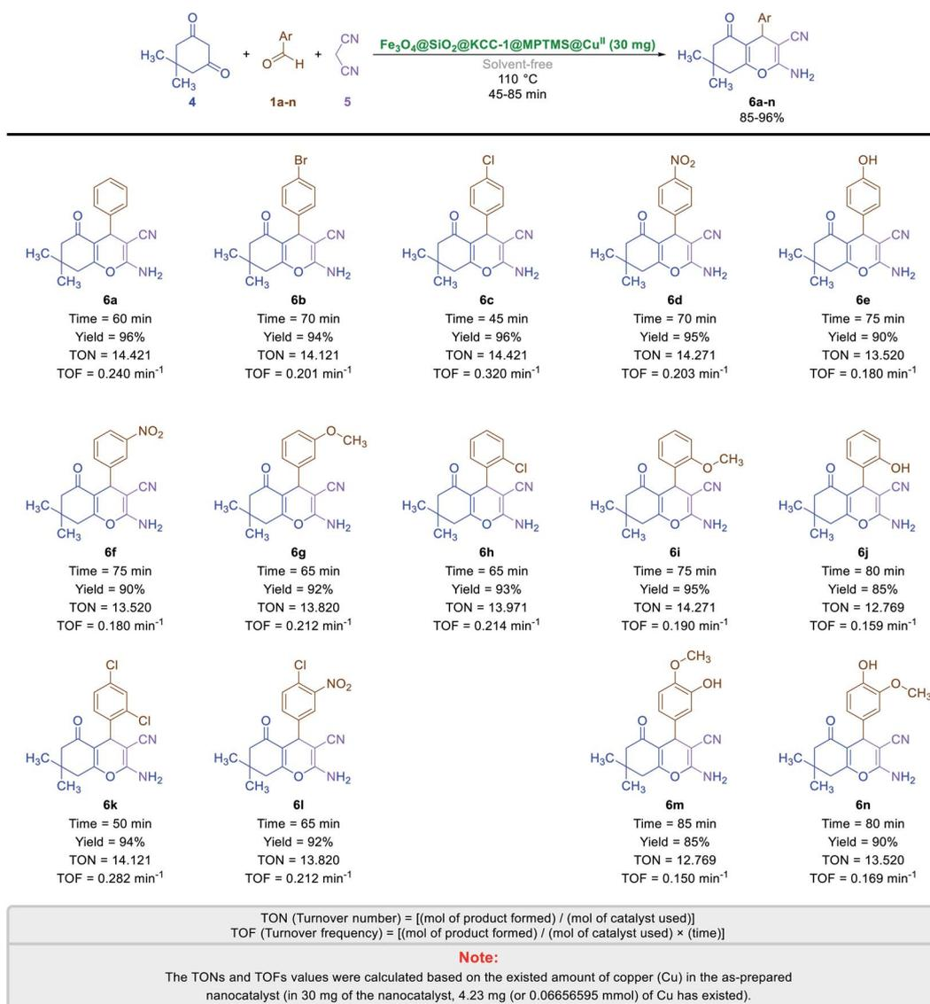
Scheme 4 Solvent-free one-pot three-component synthesis of 2-amino-4-aryl-7,7-dimethyl-5-oxo-5,6,7,8-tetrahydro-4H-chromene-3-carbonitriles (**6a–n**) catalyzed by the Fe<sub>3</sub>O<sub>4</sub>@SiO<sub>2</sub>@KCC-1@MPTMS@Cu<sup>II</sup> nanocomposite.
