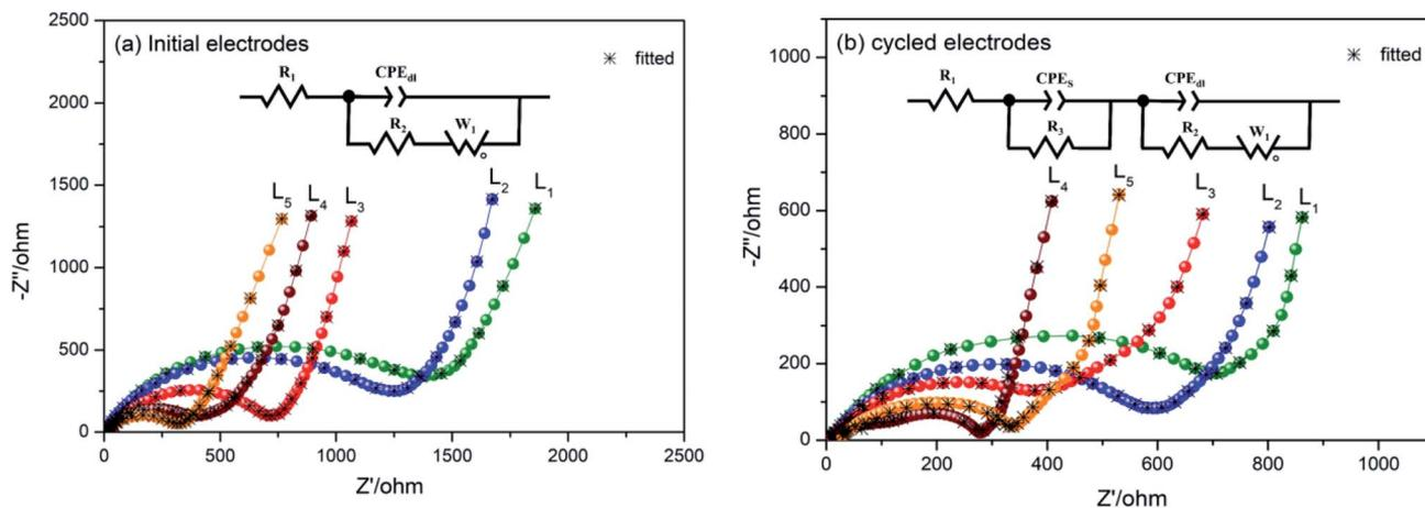
Fig. 10 Nyquist plots for electrodes and fitting curves of the laser sintering Al/Ni integrated electrodes (a) at the initial state and (b) after 3 cycles within the frequency range between 0.01 Hz and 100 kHz.
