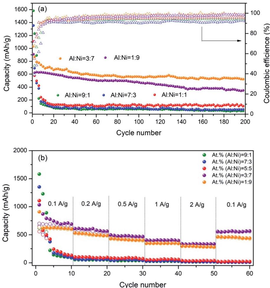
Fig. 7 (a) Cycling performances of the Al/Ni as-sintered electrodes at a current density of  $100 \text{ mA g}^{-1}$  between 0.01–2.00 V. (b) Rate capabilities of the as-sintered electrodes at various current densities from  $0.1 \text{ A g}^{-1}$  to  $2.0 \text{ A g}^{-1}$  in the potential range of 0.01–2.00 V.
