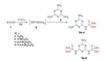
Scheme 2 One-pot sequence to bis- or tetrakis(aryl) (1,3,5-triazinyl) phosphoramidates 4 or 5 from ArOH (Ar =  $Br_nC_6H_{5-n}$ , n=0, 1–3) (1), using POCl<sub>3</sub> and melamine monomer (3).
