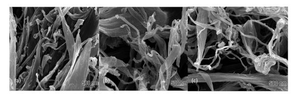
Fig. 3 SEM of LCNFs and their Mannich adducts. (a) LCNFs produced from Japanese cypress (soft wood), (b) Mannich product III with melamine monomer 3, and (c) Mannich product Vd with diphosphoramidate 5d.
