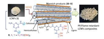
Scheme 1 Mannich reaction of (amino-1,3,5-triazinyl)mono- or diphosphoramidates (II) with LCNFs (I) and HCHO, leading to flame-retardant fabrics III-V.
