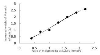
Fig. 1 The amount of the Mannich adducts with the increasing ratio of the 5a/LCNFs (mmol  $g^{-1}$ ).
