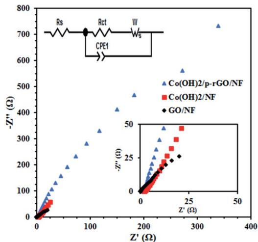
Fig. 14 Nyquist plots of the GO/NF, Co(OH)<sub>2</sub>/NF and Co(OH)<sub>2</sub>/p-rGO/NF electrodes at the open circuit potential over a frequency range of 100 kHz to 0.01 Hz. The insets show both the high frequency region and corresponding equivalent circuit.
