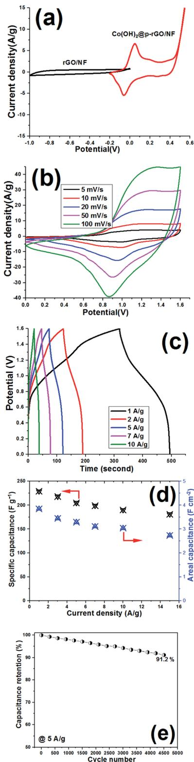
Fig. 17 Electrochemical performance of the Co(OH)<sub>2</sub>@p-rGO/NF//rGO/NF ASC device. (a) CV curves of the positive and negative electrodes at 10 mV s<sup>-1</sup>, (b) CV curves of the ASC device at different scan rates, (c) its GCD curves at different current densities, (d) the calculated specific capacities vs. current density, and (e) capacitance retention as a function of cycle number over 2500 cycles in a two-electrode system.
