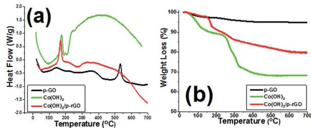
Fig. 10 TGA/DSC profiles of the prepared GO powder (p-GO), pristine  $\text{Co(OH)}_2$  and  $\text{Co(OH)}_2$ @p-rGO composite.
