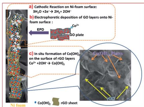
Fig. 5 Mechanisms of the electrophoretic/electrochemical deposition processes: (a) base generation step, (b) electrophoretic deposition of rGO onto NF and (c) the chemical formation of  $\text{Co}(\text{OH})_2$  on rGO.
