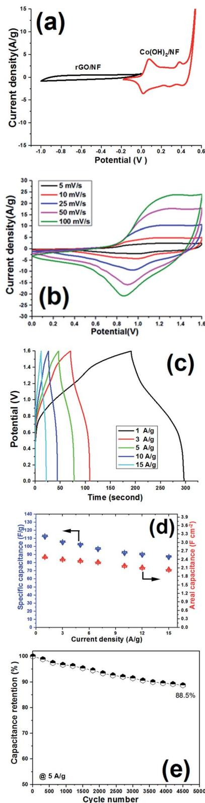
Fig. 16 Electrochemical performance of the  $\text{Co}(\text{OH})_2$ /NF//rGO/NF ASC device. (a) CV curves of the  $\text{Co}(\text{OH})_2$ /NF and rGO/NF electrodes at a scan rate of  $10 \text{ mV s}^{-1}$ , (b) CV curves of the assembled ASC device at different scan rates, (c) its GCD curves at different current densities, (d) the calculated specific capacitance vs. current load, and (e) the capacitance retention vs. cycle number at  $5 \text{ A g}^{-1}$ .
