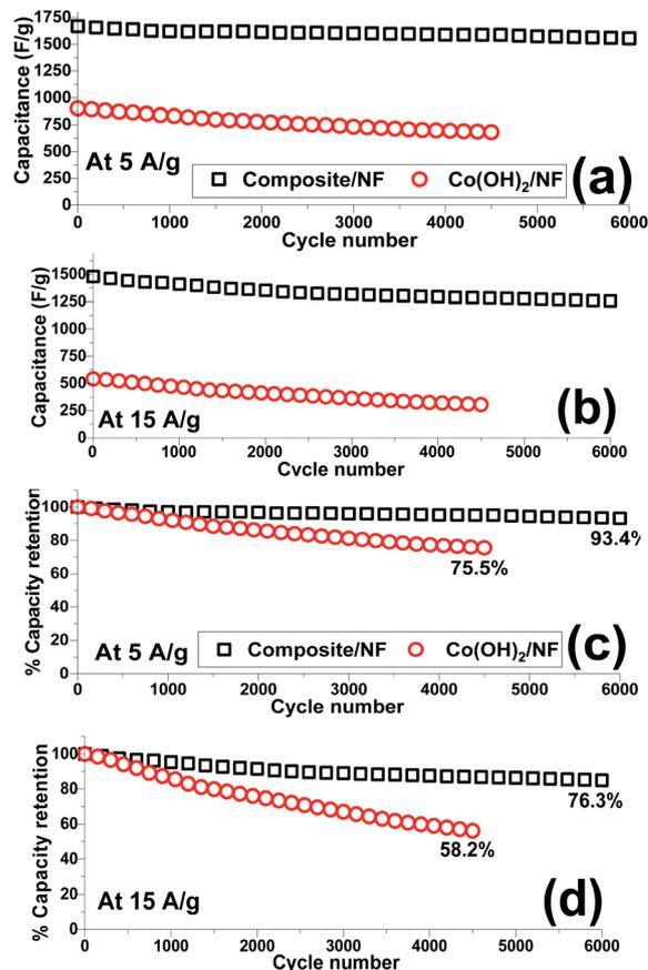
Fig. 13 Cycling data of the Co(OH)<sub>2</sub>/Ni and composite/Ni electrodes at current loads of (a and c) 5 A g<sup>-1</sup> and (b and d) 15 A g<sup>-1</sup>.
