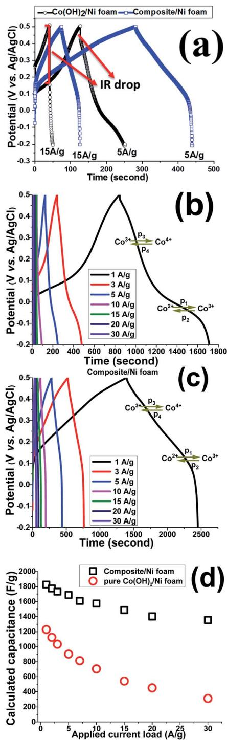
Fig. 12 (a) GCD profiles of the fabricated electrodes at currents of 5 A g<sup>-1</sup> and 15 A g<sup>-1</sup>, (b and c) GCD curves of Co(OH)<sub>2</sub>/NF and composite/NF electrodes at different current loads, and (d) calculated capacitances at various loads of 1 to 30 A g<sup>-1</sup>.
