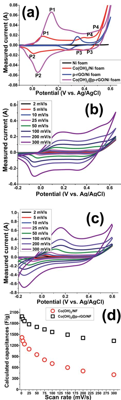
Fig. 11 (a) CVs of the fabricated electrodes (*i.e.* blank NF, Co(OH)<sub>2</sub>/NF and composite/NF) at 10 mV s<sup>-1</sup>, CV plots of the (b) Co(OH)<sub>2</sub>/NF and (c) composite/NF electrodes at the various scan rates, and (d) the calculated specific capacitances vs. the scan rate.
