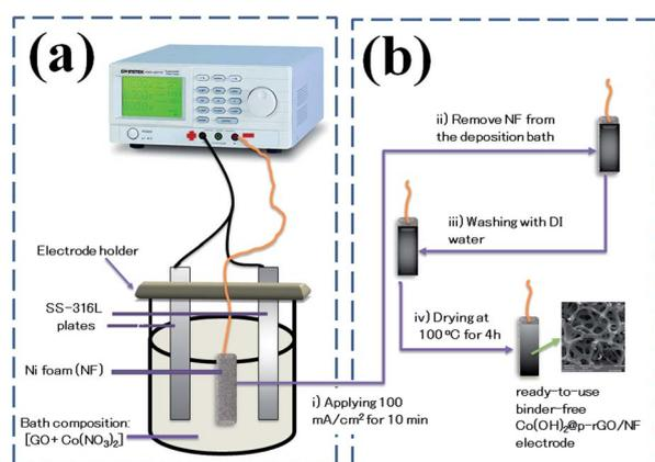
Fig. 1 Schematic of fabrication Co(OH)<sub>2</sub>@rGO onto Ni-Foam including (a) electrochemical set-up and (b) deposition procedure.
