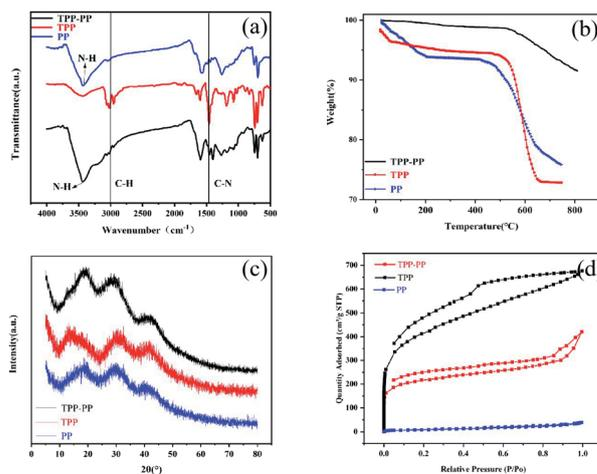
Fig. 2 (a) FT-IR spectrum of TPP-PP, TPP, PP; (b) the TG patterns of TPP-PP, TPP, PP; (c) XRD of TPP-PP, TPP, PP; (d)  $\text{N}_2$  adsorption-desorption isotherms of TPP-PP, TPP, PP at  $77 \text{ K}$ .
