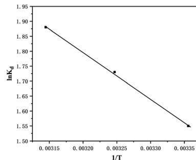
**Fig. 9** Thermodynamic curve of TPP–PP adsorption of methyl blue and linear regression graph of  $\ln K_d$  and  $1/T$ .
