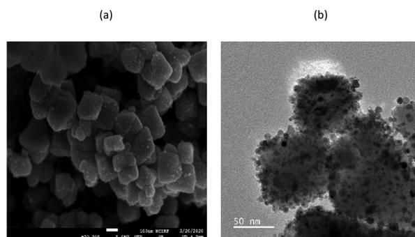
**Fig. 1** (a) SEM and (b) HR-TEM image of PdCo-Fe<sub>3</sub>O<sub>4</sub> catalyst.
