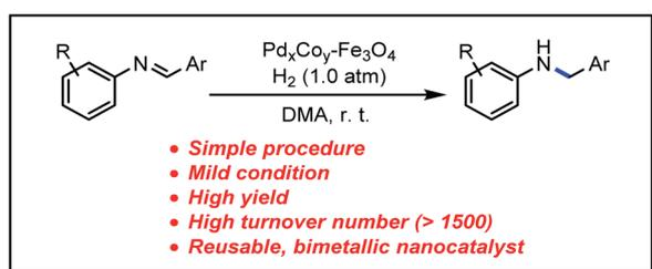
**Scheme 2** Synthesis of amines from imines using reusable PdCo-Fe<sub>3</sub>O<sub>4</sub> bimetallic catalyst under mild condition.
