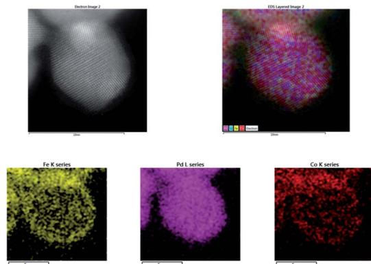
Fig. 2 STEM-EDS image of PdCo-Fe<sub>3</sub>O<sub>4</sub> catalyst.
