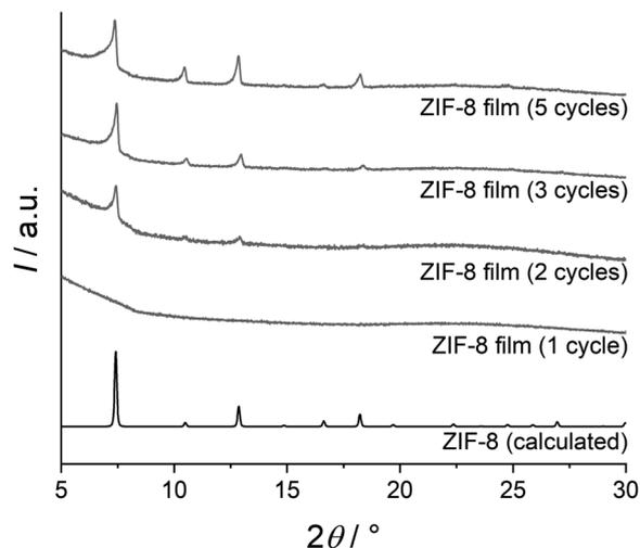
Fig. 1 XRD patterns of thin films obtained with different numbers of deposition cycles, compared with a calculated XRD pattern of ZIF-8.<sup>38</sup>
