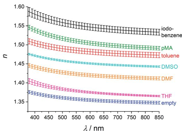
Fig. 4 Refractive index dispersion curves of guest-loaded ZIF-8 films.
