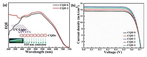
Fig. 18 (a) The external quantum efficiency (EQE) test shows an enhancement mainly in the UV region by the incorporation of CQDs. (b) I-Vcurve of DSSC at different numbers of coatings (CQD X; X is the number of N-CQDs solution coatings) (this figure has been adapted/reproduced from ref. 131 with permission from Elsevier, Copyright 2019).
