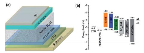
Fig. 21 (a) Organic solar cell device structure with CQDs (C in C-CQDs indicates the carbon vapour deposition method). (b) Energy level diagram of the solar cells with CQDs as ETLs and P3HT:PC $_{61}$ BM, PTB7:PC $_{61}$ BM or PTB7-Th:PC $_{71}$ BM as the active layer (This figure has been adapted/reproduced from ref. 143 with permission from Elsevier, Copyright 2016).
