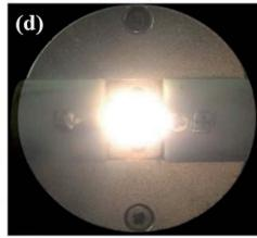
Fig. 27 (a) Images of blue, green, and red CQD phosphors under sunlight and UV light. (b) Emission spectra of the mentioned CQDs. (c) Schematic diagram of warm WLEDs consisting of blue, green and red CQDs films. (d) Photograph of the operating warm WLED with brilliant warm white emission (this figure has been adapted/reproduced from ref. 166 with permission from Wiley-VCH, Copyright 2017).
