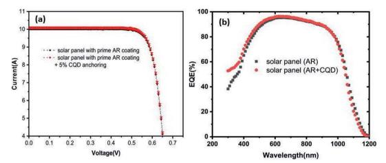
Fig. 19 (a) I-V characteristics of solar cells (with and without CQDs) exhibiting an increase in  $I_{SC}$  in the presence of CQDs. (b) Enhanced EQE of solar cells in the presence of CQDs in the UV region (this figure has been adapted/reproduced from ref. 134 with permission from Elsevier, Copyright 2022).
