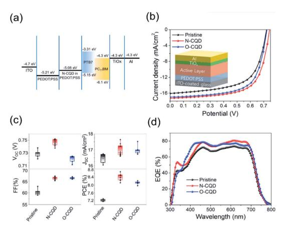
Fig. 23 OPV device performance and characterization. (a) Energy band diagram of the OPV device. (b) Current vs. potential (J-V) curves (inset: OPV device with the structure ITO/PEDOT:PSS/active layer/TiO<sub>x</sub>/Al). (c) Photovoltaic response, and (d) EQE spectra of OPV devices (this figure has been adapted/reproduced from ref. 149 with permission from Elsevier, Copyright 2021).
