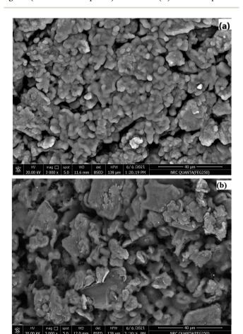
Fig. 3 SEM images for PDCTETA-SPE surface (a) before and (b) after soaking in  $1.0\times10^{-3}$  mol L<sup>-1</sup> Ce(iii) ions solution.
