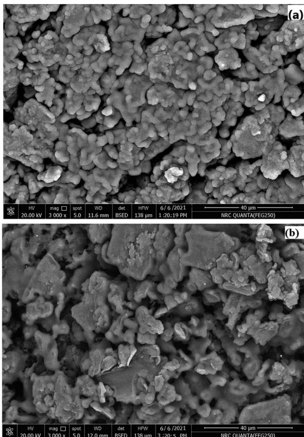
Fig. 3 SEM images for PDCTETA-SPE surface (a) before and (b) after soaking in 1.0 × 10<sup>-3</sup> mol L<sup>-1</sup> Ce(III) ions solution.
