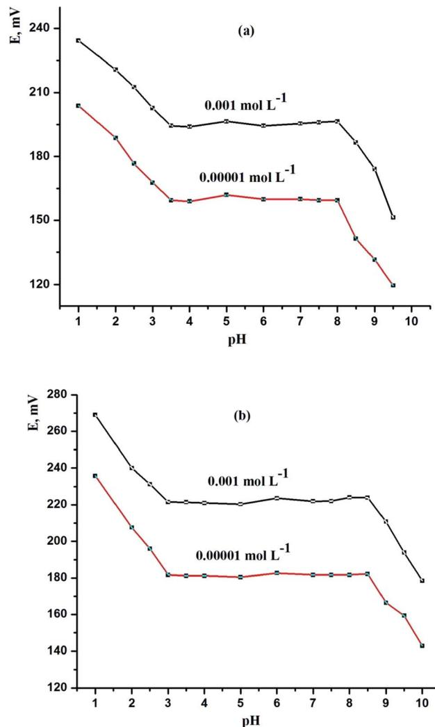
Fig. 5 Effect of pH of the test solution on the performance characteristics of (a) CPS (sensor IV) and (b) SPS (sensor VIII) at  $T = 25^\circ C$  and  $[Ce(III)] = 1 \times 10^{-3}$  and  $1 \times 10^{-5}$  mol  $L^{-1}$ .
