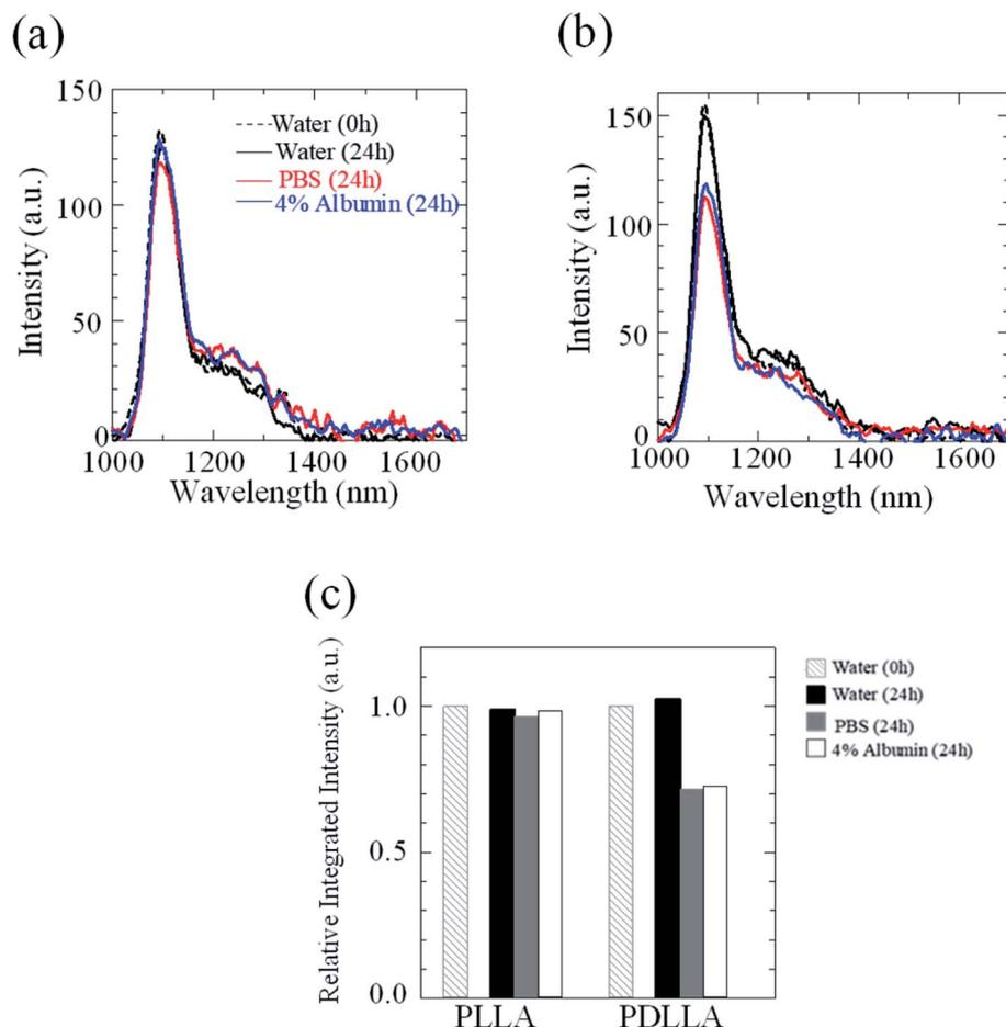
Fig. 5 Effect of dispersion media on OTN-NIR fluorescence intensity of the IR-1061-loaded polymer micelles of PEG-*b*-PLA. Fluorescence spectra for IR-1061-loaded PEG-*b*-PLLA (a) and PEG-*b*-PDLLA (b) polymer micelles dispersed in indicated media for 24 h. Integrated intensities (1000–1400 nm) are also shown for IR-1061-loaded PEG-*b*-PLLA and PEG-*b*-PDLLA polymer micelles dispersed in indicated media for 24 h (c).
