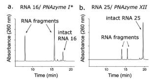
Fig. 7 IEX-HPLC chromatograms showing the extent of cleavage of a 33-fold excess of (a) RNA 16 (14mer) and (b) RNA 25 (18mer) (100  $\mu$ M) by their corresponding PNAzymes (3  $\mu$ M) after 6 h of incubation in the presence of Zn<sup>2+</sup> (100  $\mu$ M) at 37 °C, pH 7. \*The data shown in panel (a) has been previously reported by Luige *et al.*<sup>15</sup>
