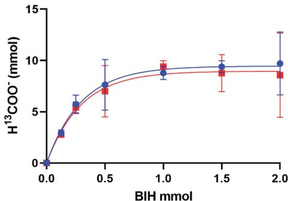
Fig. 3 A plot of  $\text{H}^{13}\text{COO}^-$  (mmol) vs. BIH (mmol) upon blue light (450–460 nm) irradiation of **1** (blue circles,  $R^2 = 0.9932$ ) and **2** (red squares,  $R^2 = 0.9864$ ).  $\text{H}^{13}\text{COO}^-$  increased with an exponential curve fit and reached a plateau at  $y = 9.45$  and  $8.96$  mmol  $\text{H}^{13}\text{COO}^-$ , respectively.
