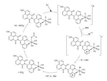
Fig. 4 Proposed hydride mechanism of  $CO_2$  reduction to formate *via* 1 or 2. X = Cl or Br, Sol = DCM or MeOH.
