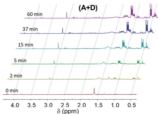
Fig. 6 Proton NMR spectra obtained for the (A + D) formulation during irradiation.
