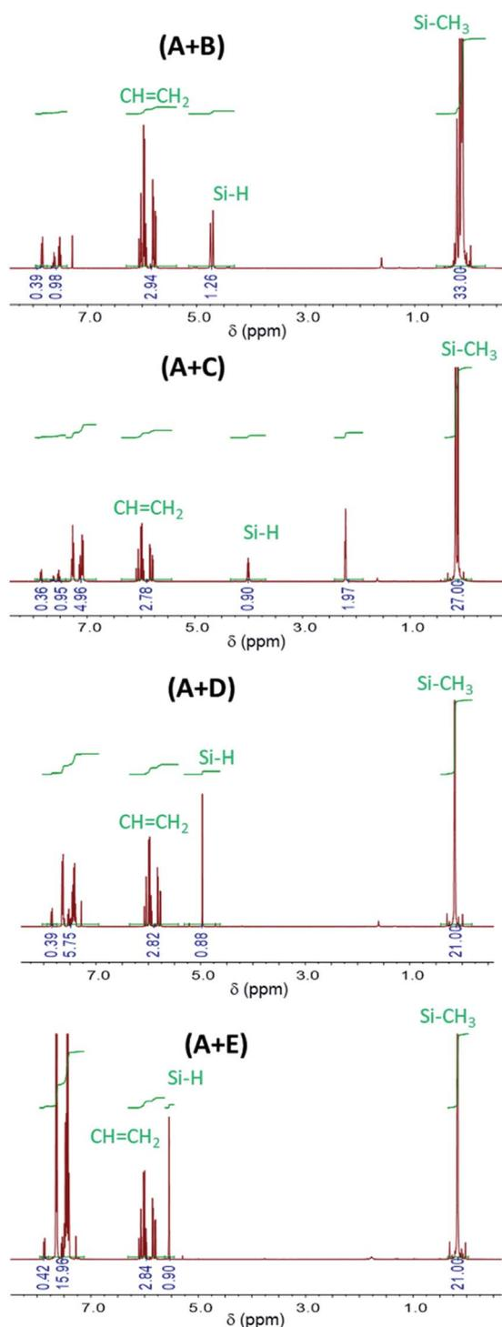
Fig. 1  $^1\text{H}$ -NMR spectra of (A + B), (A + C), (A + D) and (A + E) formulations prior to UV irradiation ( $t = 0$ ).
