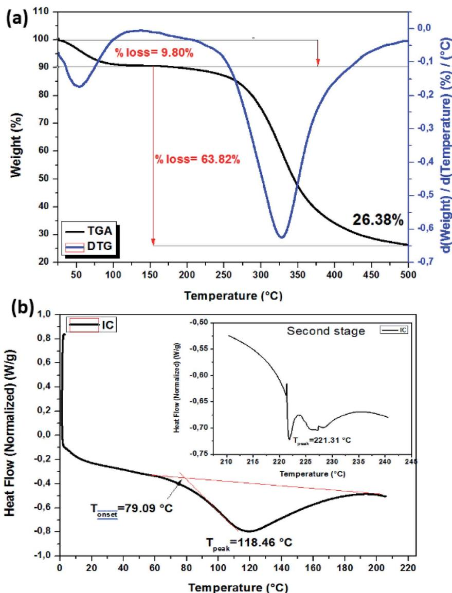
Fig. 6 (a) TGA and DTG curves of insoluble collagen (IC) in the range of 25 °C to 500 °C. (b) DSC curve of insoluble collagen (IC) in the range of 0 °C to 220 °C (inset: the second stage in the range of 220 °C to 245 °C).
