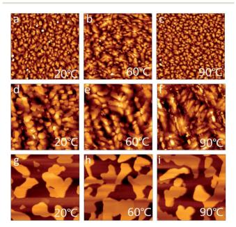
Fig. 5 AFM images (5  $\mu$ m  $\times$  5  $\mu$ m) of the thin films of DIN (a-c), DSN (d-f) and DPEN (g-i) deposited at different temperatures.
