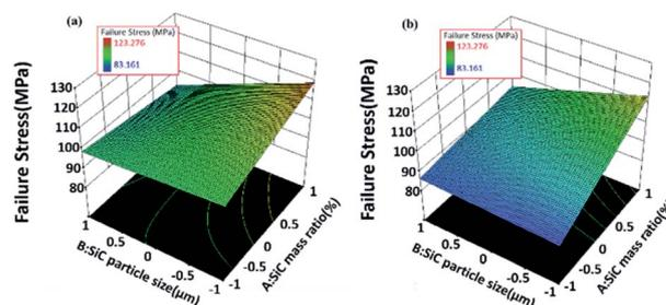
Fig. 9 Response surface plots presenting the dependence of failure stress ( $S$ ) on the SiC mass ratio ( $A$ ) and the SiC particle size ( $B$ ) for the (a) minimum Al particle size ( $C = -1$ ) and (b) maximum Al particle size ( $C = 1$ ).
