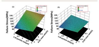
Fig. 10 Response surface plots presenting the dependence of failure stress (S) on the SiC mass ratio (A) and the Al particle size (C) for the (a) minimum SiC particle size (B=-1) and (b) maximum SiC particle size (B=1).
