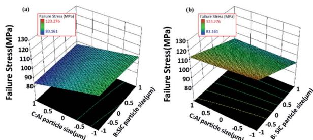
Fig. 11 Response surface plots presenting the dependence of failure stress ( $S$ ) on the SiC particle size ( $B$ ) and the Al particle size ( $C$ ) for the (a) minimum SiC mass ratio ( $A = -1$ ) and (b) maximum SiC mass ratio ( $A = 1$ ).
