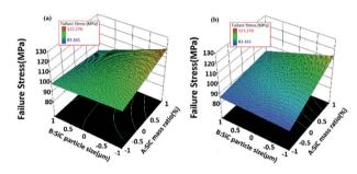
Fig. 9 Response surface plots presenting the dependence of failure stress (S) on the SiC mass ratio (A) and the SiC particle size (B) for the (a) minimum Al particle size (C=-1) and (b) maximum Al particle size (C=1).
