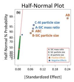
Fig. 4 The half-normal plot of responses (a) S and (b) P.
