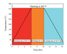
Fig. 2 The sinter temperature curve of reactive materials.
