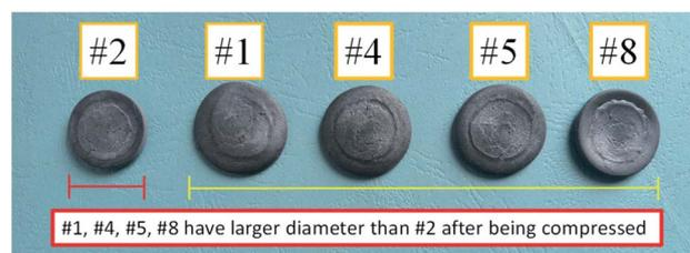
Fig. 13 Top view of specimens after compression.
