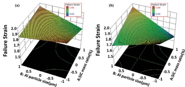
Fig. 14 Response surface plots presenting the dependence of failure strain ( $P$ ) on the SiC mass ratio ( $A$ ) and the SiC particle size ( $B$ ) for the (a) minimum Al particle size ( $C = -1$ ) and (b) maximum Al particle size ( $C = 1$ ).
