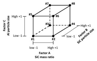
Fig. 1 Geometric view of full 2<sup>3</sup> factorial design
