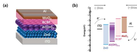
Fig. 4 Schematic illustrations of (a) device architecture and (b) energy band diagram of  $\text{Al}(\text{OH})_{3-x}$  based LED with inverted device structure of [ITO/ZnO nanoparticle films (40 nm)/emissive active layers/BCBP (50 nm)/ $\text{MoO}_3$  (10 nm)/Al (100 nm)]. ZnO and emissive  $\text{Al}(\text{OH})_{3-x}$  layers were prepared by spin-casting and BCBP,  $\text{MoO}_3$ , and Al were thermally evaporated on top of the spun-cast ZnO/ $\text{Al}(\text{OH})_{3-x}$  layers.
