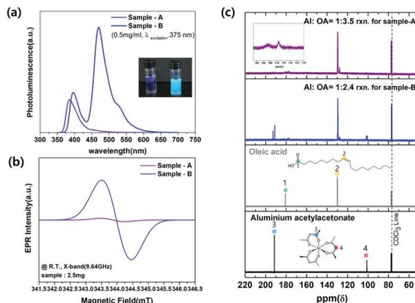
Fig. 3 (a) PL spectra of Sample-A and B at the same concentrations ( $0.5\text{ mg mL}^{-1}$ ) dispersed in hexane. The inset images of samples emitted under  $365\text{ nm}$  UV light at room temperature. (b) X-band ( $9.64\text{ GHz}$ ) EPR spectra of Sample-A (violet color) and -B (blue color) powder at room temperature. (c)  $^{13}\text{C}$  NMR spectra of initiators before synthesis of Sample-A or B, oleic acid, and aluminum acetylacetonate (from the top spectrum down).
