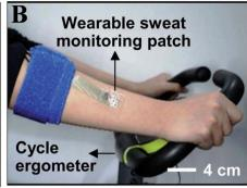
Fig. 9 (A) Optical camera image of the disposable strip-type sensors connected to a zero insertion force (ZIF) connector. (B) Optical camera image of the subject using a cycle ergometer for sweat generation with the wearable patch on the subject's arm (Science advances).<sup>123</sup>
