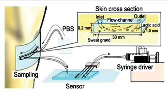
Fig. 5 Lactic acid monitoring system showing schematic representation.<sup>86</sup> (Wiley Periodicals, Inc).
