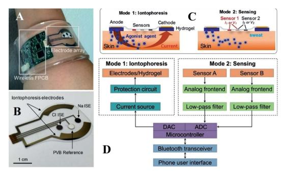
Fig. 2 (A) Self-contained sensing and sweat extraction platforms. (B) Cl<sup>-</sup> and Na<sup>+</sup> measuring iontophoresis and sweat sensor electrodes (C) schematic of sensing modes and iontophoresis (D) system-level block diagram of sensing circuits and iontophoresis<sup>73</sup> (Copyright 2017, National Academy of Science).
