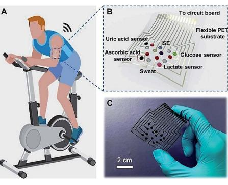
Fig. 6 Silk NCT based wearable sweat analysis patch (A and B). Graphical illustration of human skin mounts for sweat analysis patch and integration of multiplex electrochemical sensor array in the patch (C) photographic representation of wearable sweat patch analysis.<sup>83</sup> (Photo credit: Wenya He, Tsinghua University Wenya He *et al.* Sci Adv 2019).
