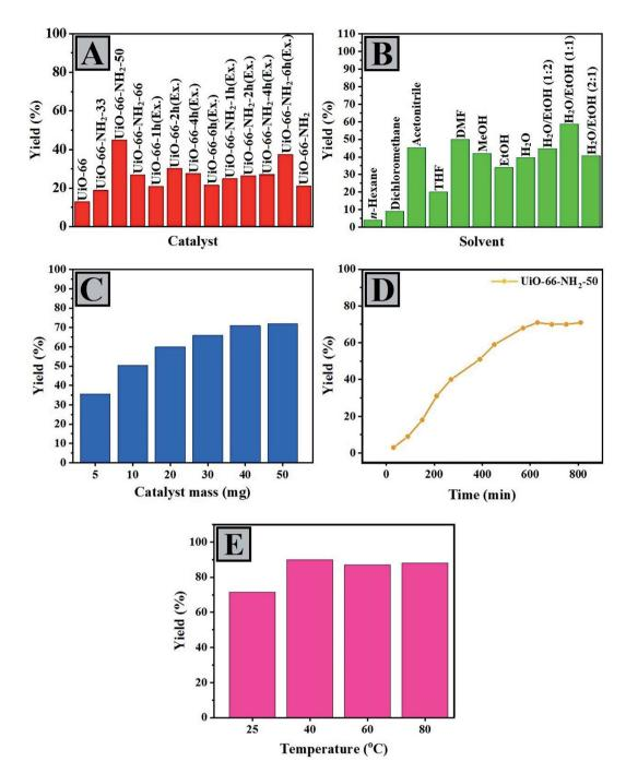
Fig. 3 Optimization of the catalysts, solvent, catalyst loading, time and temperature (A-E) for the Knoevenagel condensation of aldehydes.
