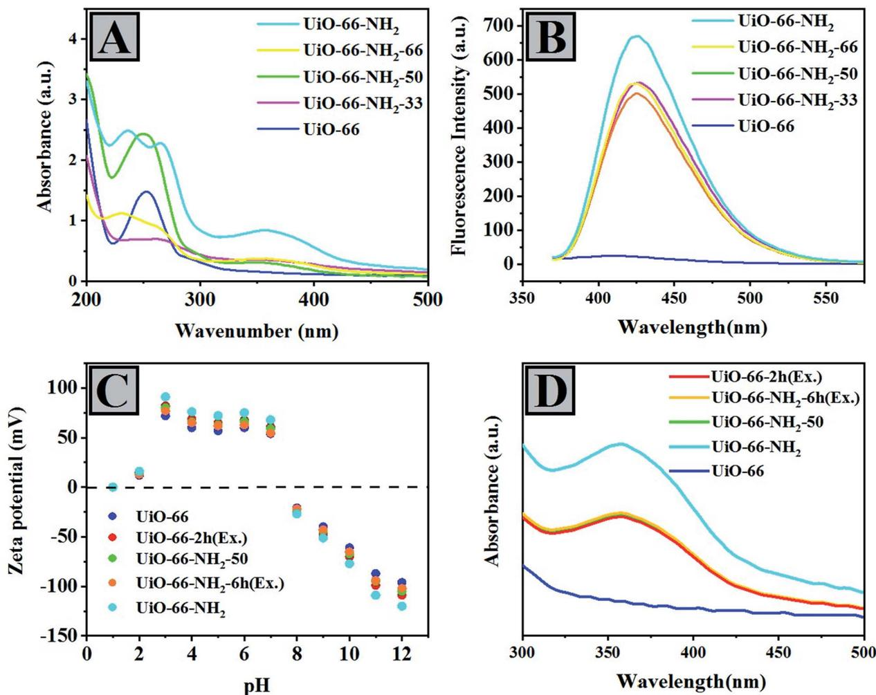
Fig. 2 (A) UV-vis DRS and (B) PL spectroscopy of mixing-ligand prepared compounds. (C) Zeta potential and (D) UV-vis comparative analysis of 2-aminoterephthalic acid in 1 M NaOH solution.
