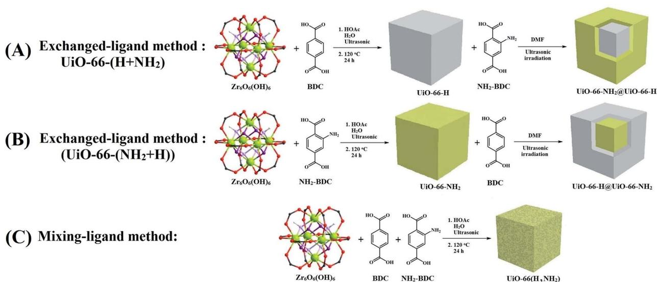
Scheme 1 Synthesis of catalytic systems.
