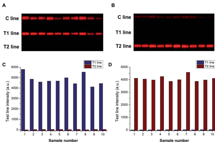
Fig. 4 Repeatability of the duplex RT-PCR-combined LFA. Images of 10 test strips for 10<sup>4</sup> copies per μL of (A) SARS-CoV-2 and (B) IBV. Corresponding fluorescence intensities of (C) SARS-CoV-2 and (D) IBV.
