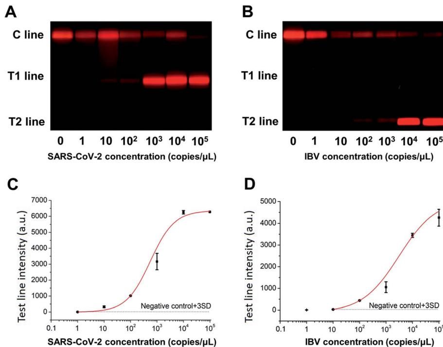
Fig. 3 Images of test strips at different concentrations of (A) SARS-CoV-2 and (B) IBV in the range of 1 to 10<sup>5</sup> copies per μL. Corresponding fluorescence intensities and fitting curves on the test lines of (C) SARS-CoV-2 and (D) IBV. Error bars represent the standard deviation of three repetitive experiments.
