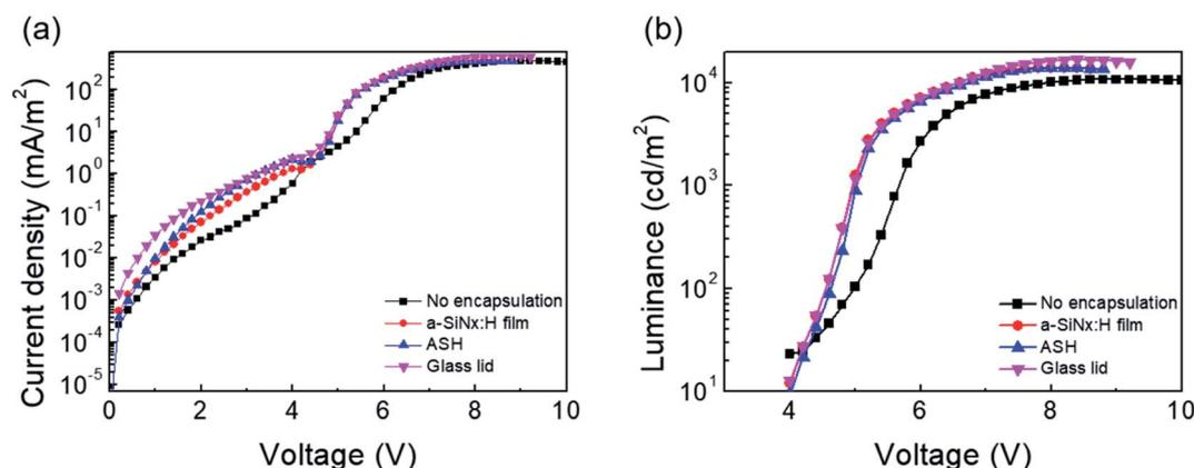
Fig. 4 (a) Luminance–voltage characteristic curve and (b) current density–voltage characteristic curve of the QD-LEDs without encapsulation and QD-LEDs encapsulated with the a-SiN<sub>x</sub>:H film, the ASH films, and glass lid.
