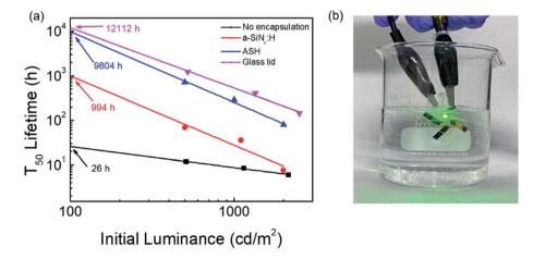
Fig. 6 (a) The estimated  $T_{50}$  of the QD-LEDs without encapsulation, and encapsulated QD-LEDs with the a-SiN<sub>x</sub>:H film, the ASH film, and glass lid. (b) Photograph of the encapsulated QD-LEDs with the ASH film immersed in water.
