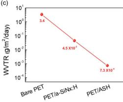
Fig. 2 (a) Optical transmittance spectra of the bare PET substrate, PET/a-SiN<sub>x</sub>:H film, and PET/ASH film. The inset shows photograph of the KIST logo under a PET/ASH barrier. (b) The normalized conductance curve of bare PET, PET/a-SiN<sub>x</sub>:H film, and PET/ASH film. The inset displays a schematic of the Ca sensor. (c) The calculated WVTR values of bare PET, PET/a-SiN<sub>x</sub>:H film and PET/ASH film from the Ca test.
