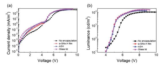
Fig. 4 (a) Luminance-voltage characteristic curve and (b) current density-voltage characteristic curve of the QD-LEDs without encapsulation and QD-LEDs encapsulated with the a-SiN<sub>x</sub>:H film, the ASH films, and glass lid.
