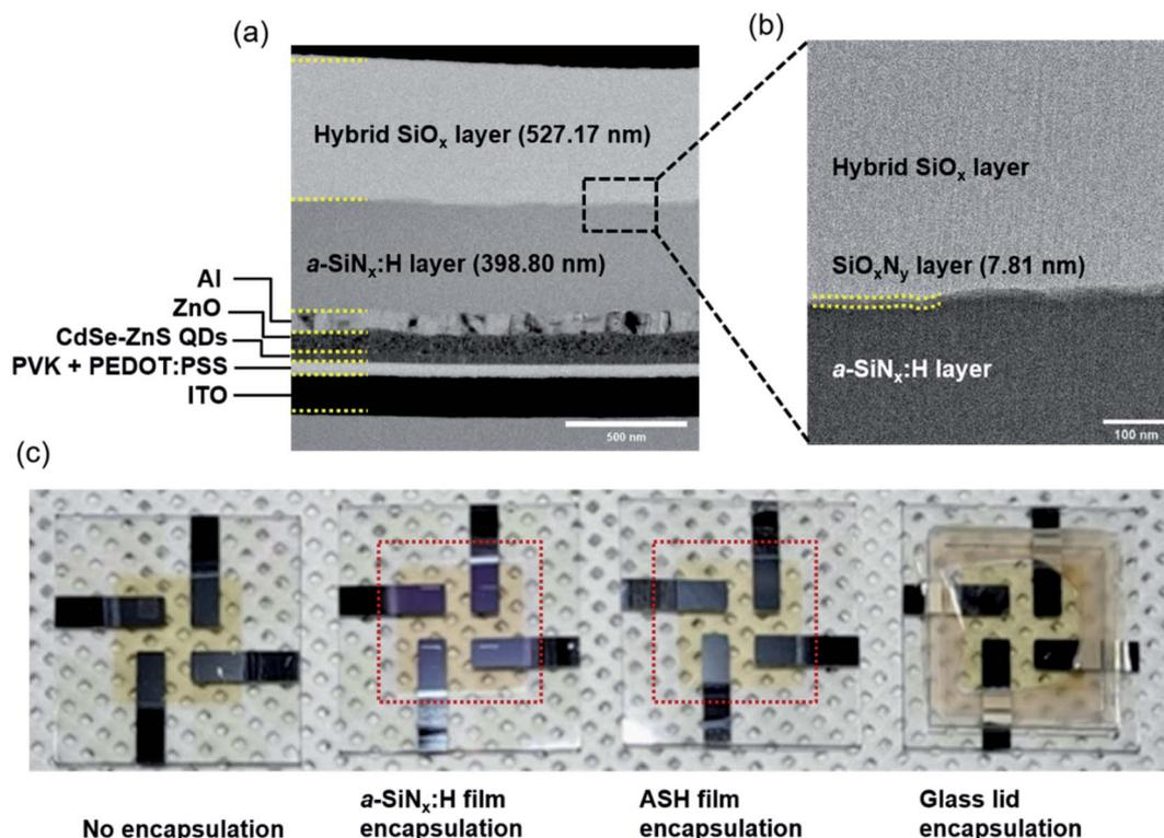
Fig. 3 (a) Cross-sectional TEM images of encapsulated QD-LEDs with the ASH film and (b) the magnified view of the ASH layer. (c) Photograph of QD-LEDs without encapsulation and encapsulated with the a-SiN<sub>x</sub>:H film, the ASH film, and glass lid.
