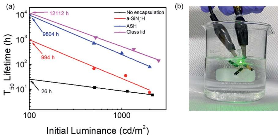
Fig. 6 (a) The estimated T<sub>50</sub> of the QD-LEDs without encapsulation, and encapsulated QD-LEDs with the a-SiN<sub>x</sub>:H film, the ASH film, and glass lid. (b) Photograph of the encapsulated QD-LEDs with the ASH film immersed in water.
