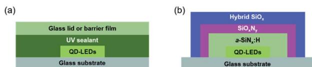
Fig. 1 (a) Schematic of conventional glass lid encapsulated QD-LEDs and (b) the ASH films encapsulated QD-LEDs.
