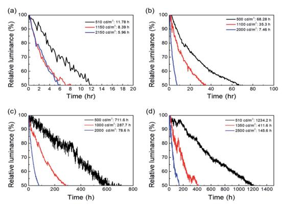
Fig. 5 (a) Operational lifetimes of the QD-LEDs without encapsulation, and (b) encapsulated QD-LEDs with the a-SiN $_x$ :H film, (c) the ASH films, and (d) glass lid.
