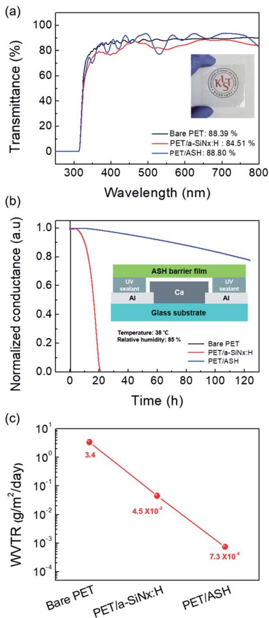
Fig. 2 (a) Optical transmittance spectra of the bare PET substrate, PET/a-SiN<sub>x</sub>:H film, and PET/ASH film. The inset shows photograph of the KIST logo under a PET/ASH barrier. (b) The normalized conductance curve of bare PET, PET/a-SiN<sub>x</sub>:H film, and PET/ASH film. The inset displays a schematic of the Ca sensor. (c) The calculated WVTR values of bare PET, PET/a-SiN<sub>x</sub>:H film and PET/ASH film from the Ca test.
