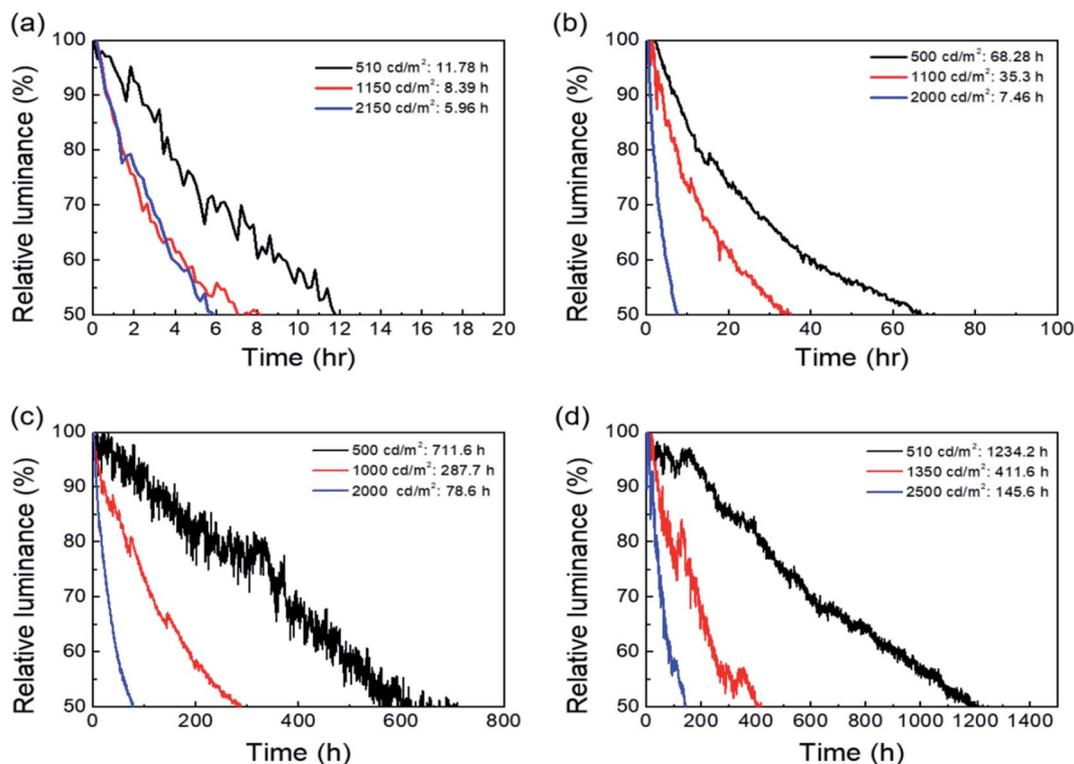
Fig. 5 (a) Operational lifetimes of the QD-LEDs without encapsulation, and (b) encapsulated QD-LEDs with the a-SiN<sub>x</sub>:H film, (c) the ASH films, and (d) glass lid.
