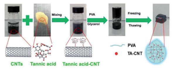
Fig. 4 The preparation of TA-CNT-glycerol-PVA hydrogel for moist-electric generation. Reproduced from ref. 54 with permission from the Royal Society of Chemistry, copyright 2020.
