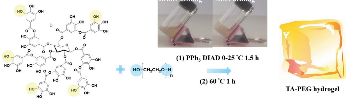
Fig. 12 Direct PEGylation of TA under mild conditions to construct a TA-PEG hydrogel. Reproduced from ref. 122 with permission from the Royal Society of Chemistry, copyright 2021.
