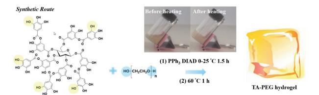
Fig. 12 Direct PEGylation of TA under mild conditions to construct a TA-PEG hydrogel. Reproduced from ref. 122 with permission from the Royal Society of Chemistry, copyright 2021.
