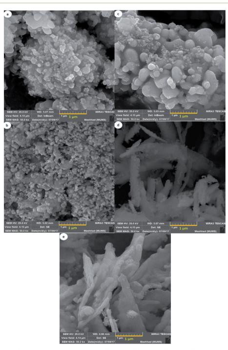
Fig. 2 FE-SEM image of NaY(WO<sub>4</sub>)<sub>2</sub> nanostructures fabricated by (a) glucose, (b) fructose, (c) lactose, (d) cellulose, and (e) starch as capping agents.
