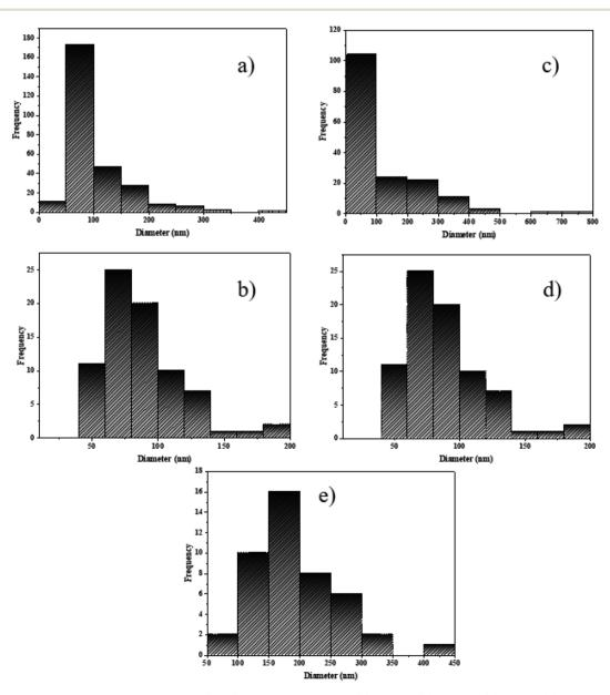
Fig. 3 The particle size distribution histogram of NaY(WO<sub>4</sub>)<sub>2</sub> samples prepared by (a) glucose, (b) fructose, (c) lactose, (d) cellulose, and (e) starch using Digimizer as the image analyser.
