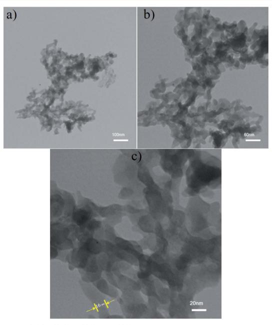
Fig. 4 TEM images of NaY(WO<sub>4</sub>)<sub>2</sub> at (a) 100 nm, (b) 60 nm, and (c) 20 nm scale bar fabricated by fructose as the optimum sample (S2). Particle shape of the NaY(WO<sub>4</sub>)<sub>2</sub> is identified by TEM images.
