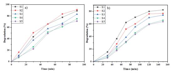
Fig. 8 Photocatalytic elimination of Rd.B below the lighting of (a) UV, and (b) Vis on NaY(WO<sub>4</sub>)<sub>2</sub> nanostructures (sample S1–S6).
