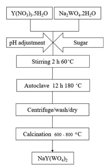
Scheme 1 Schematic for NaY(WO<sub>4</sub>)<sub>2</sub> synthesis using the precursors.
