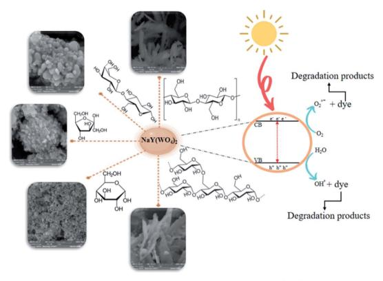
Scheme 2 The graphical mechanism for the synthesis and photodegradation performance of NaY(WO<sub>4</sub>)<sub>2</sub> nanoparticles.
