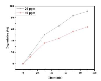
Fig. 9 The effect of the Rd.B dosage on the photocatalytic activity of  $NaY(WO_4)_2$  nanoparticles (sample S2).
