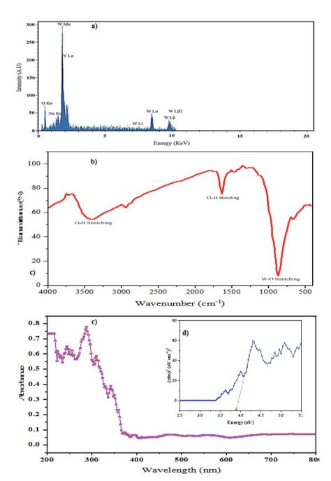
Fig. 6 (a) EDS result of NaY(WO<sub>4</sub>)<sub>2</sub> fabricated by fructose as the optimum sample S2, (b) FT-IR spectrum of the as-synthesized NaY(WO<sub>4</sub>)<sub>2</sub> nanoparticles, (c) Drs spectrum of the sample S2, and (d) curve  $(\alpha h \nu)$ 2 against  $h \nu$  of sample S2.
