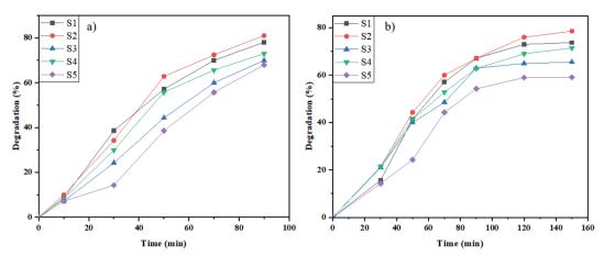
Fig. 7 Photocatalytic elimination of M.O below the lighting of (a) UV, and (b) Vis on NaY(WO<sub>4</sub>)<sub>2</sub> nanostructures (sample S1–S6).
