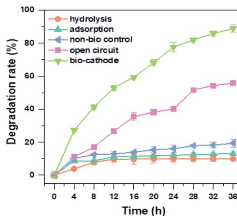
Fig. 2 TEC degradation processes in different units (degradation condition:  $C_{\text{TEC}} = 10 \text{ mg L}^{-1}$ , NaAc as carbon source,  $C_{\text{carbon source}} = 0.5 \text{ g L}^{-1}$ , aeration strength =  $12 \text{ L h}^{-1}$ ).
