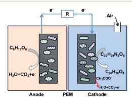
Mechanism of TEC degradation on MFC bio-cathode.
