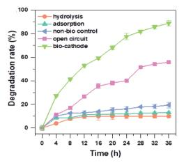
Fig. 2 TEC degradation processes in different units (degradation condition:  $C_{\text{TEC}} = 10 \text{ mg L}^{-1}$ , NaAC as carbon source,  $C_{\text{carbon source}} =$  $0.5 \text{ g L}^{-1}$ , aeration strength = 12 L h<sup>-1</sup>).
