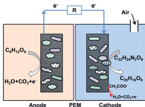
Fig. 4 Mechanism of TEC degradation on MFC bio-cathode.
